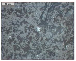
Figure 17- Subhedral magnetite in the center.
