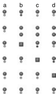
Fig. 13. Possible configuration of hydroxyl ions, peroxide or oxide ions and vacancies in the channel along the crystallographic c-axis in hydroxyl-peroxy apatite. O, H atoms and vacancies are presented by large gray circles, small open circles and gray squares, respectively. Filled small circles represent H atoms perturbed by the incorporation of peroxide ions [85].
