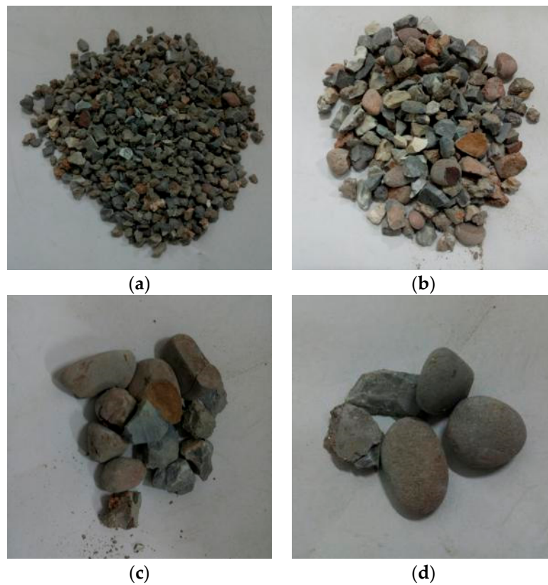
Figure 8. Concrete particles after slow heating up to 800 °C and sieving (impact speed 8.6 m/s), water cooling. (a) 5 mm (51.97%); (b) 10 mm (26.44%); (c) 16 mm (8.2%); (d) 20 mm (13.29%).
