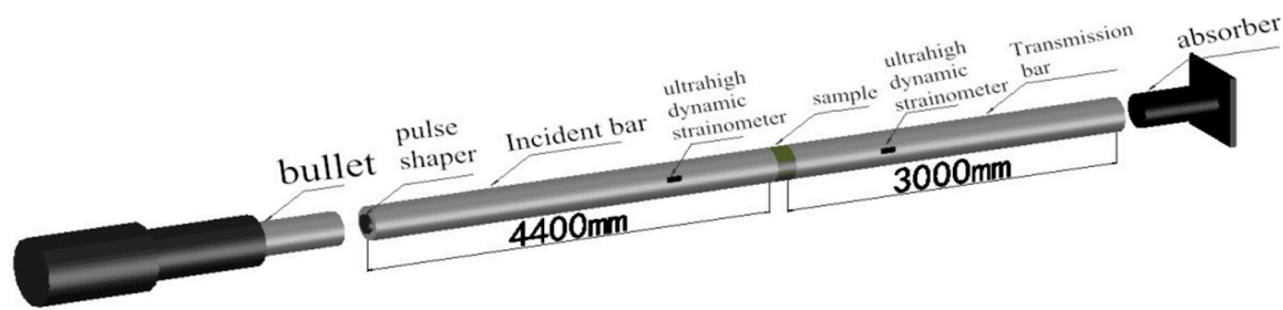
Figure 3. SHPB test system structure.
