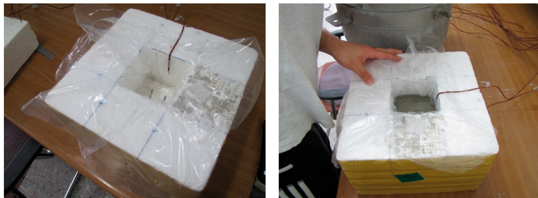
Figure 2. Set-up for semi-adiabatic temperature rise testing.
