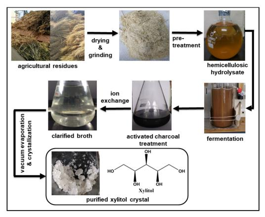
**Figure 3.** Processing of lignocellulosic biomass for xylitol production. Agricultural residues are dried and grounded to obtain coarse powder, which is treated with chemical/biological reagents to obtain hemicellulosic hydrolysate. Microorganisms ferment the hydrolysate to various byproducts such as xylitol. After fermentation, broth is treated with activated charcoal and ion exchange resins to remove the contaminants, and xylitol crystals are obtained after lyophilization of clarified broth.
