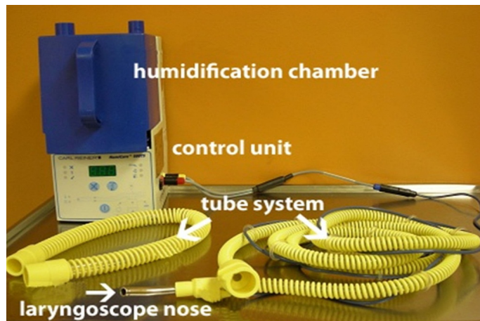
Figure 15. Device for moistening and warming-up of the respiration gas. The central unit (white) incorporates the electronic control unit. The humidifying chamber (blue) for single or multiple use is fixed at the central unit. The tubing system (yellow) is split into a short tube which transports the ventilation gas coming from the respirator to the humidifying chamber, and in a long tube which transports the now moistened and warmed-up gas from the humidifier chamber to the jet laryngoscope. The distal part of the long tube is metallic and is connected to the jet laryngoscope.
