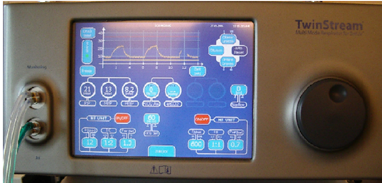
Figure 11. Jet respirator for the combined high-frequent and low-frequent jet ventilation (Twin Stream™ multimode respirator, Carl Reiner Ltd. Company with limited liability, Vienna, Austria). The continuous airway pressure is displayed in the left upper corner. The top right part shows the adjustable pressure limitation. In the middle left the digital airway pressure and in the center of the display the inspiratory oxygen concentration is displayed. On the lower left side the low-frequency jet unit can be seen and on the right there is the high-frequency jet unit.
