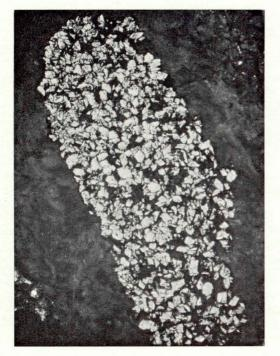
Fig. 2. Aggregate of cassiterite crystals in rankamaite.  $40 \times .$
