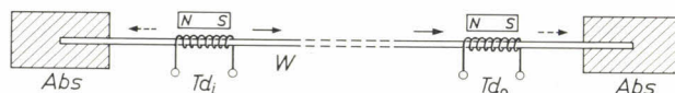
Fig. 1. Wire delay line. The electrical input signal fed to the input transducer Td_i launches an acoustic wave down the wire W ; this wave induces a voltage in the coil of the output transducer Td_o . Reflections from the ends of the wire are prevented by the use of absorbent terminations Abs .
