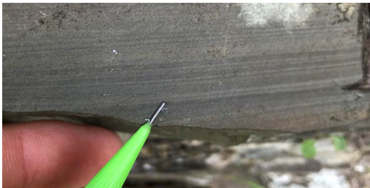
Figure 3.32 Willy Scrow Trilobitic Mudstone . GR: 27620, 96104. Typical lamination observed throughout the formation. Alternating dark grey and grey bands with 2mm of thickness.
