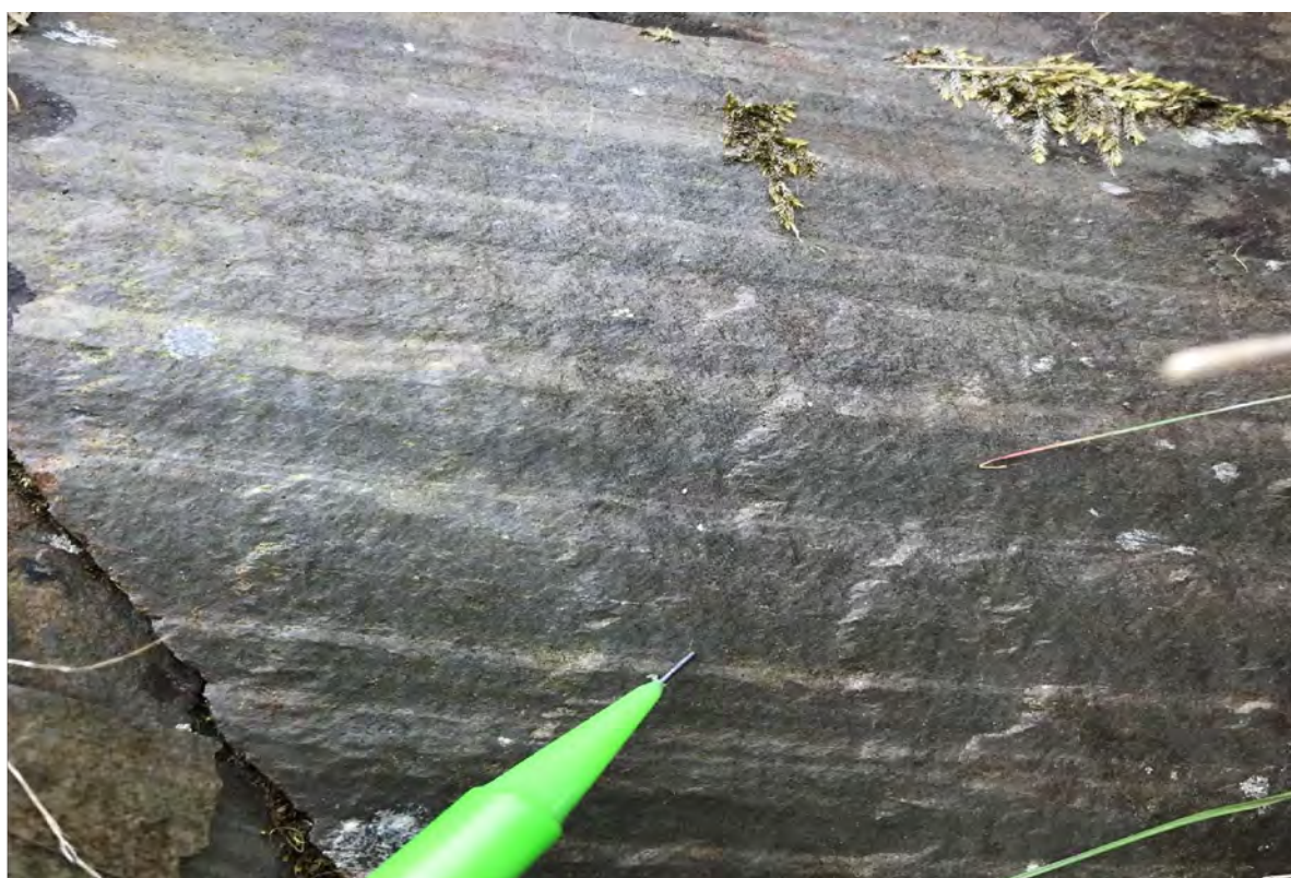
Figure 3.59 Torver Black Mudstone GR: 27764, 93654. Bands of lamination within the TBM can range between 1 and 20mm thickness.
