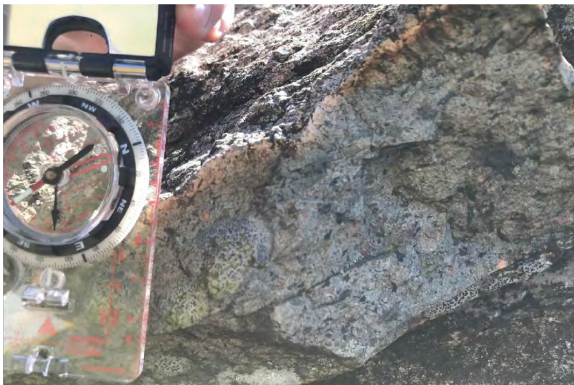
Figure 3.8 Buck Pike Tuff and Clastic Fmt. GR: 29085, 97953. A field photo of the internal lithology of the ignimbrite member. Lense shaped fiamme describing eutaxitic textures are abundant, commonly 1cm in width.
