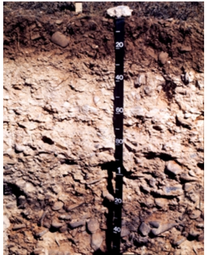
Photo 6.—A mollic epipedon approximately 25 cm thick over a calcic horizon in a soil from Idaho.
