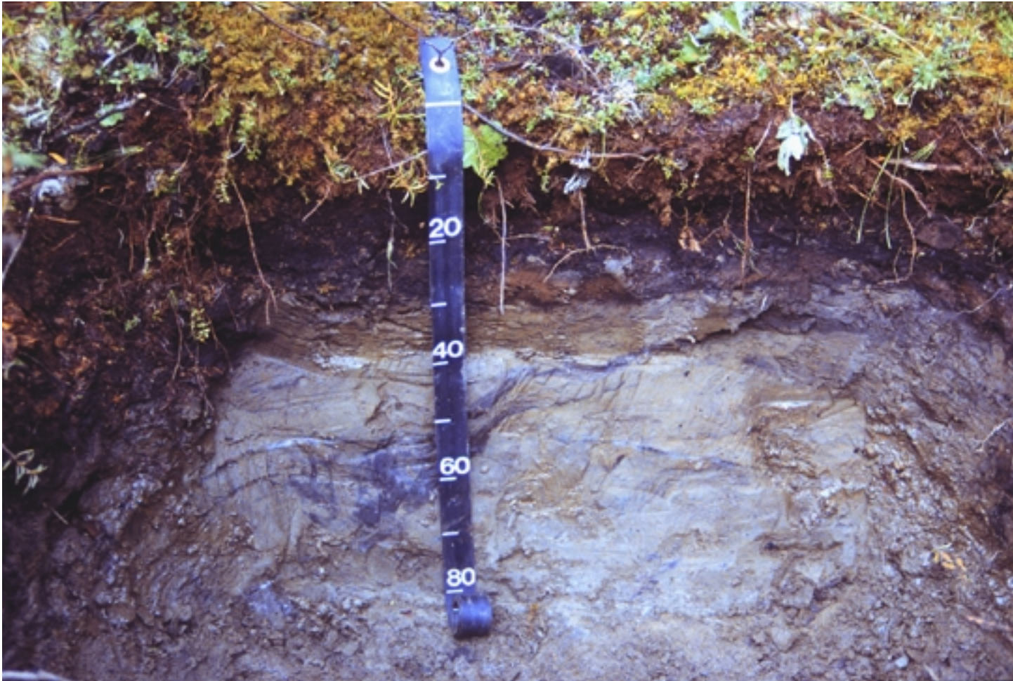
Photo 37.—A Turbel from the Yukon Territory with cryoturbation in the subsoil.
