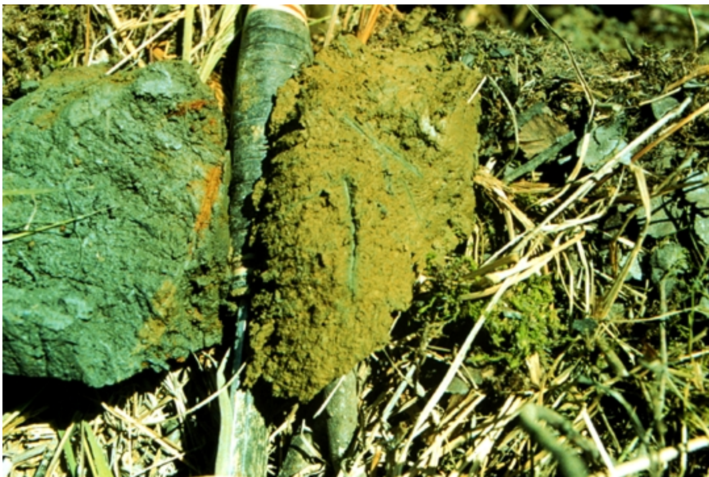
Photo 36.—Peds from a gleyed horizon and the horizon directly below.
