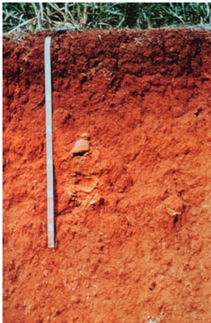
Photo 8.—An ochric epipedon from an Oxisol in Hawaii. The ochric epipedon has high value and chroma.
