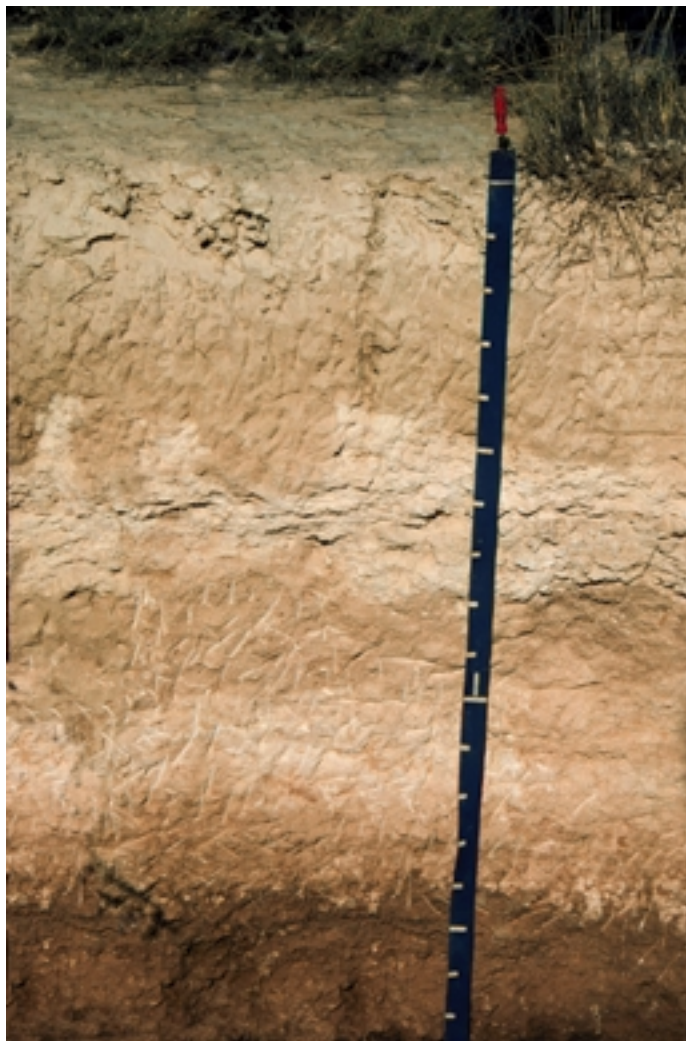
Photo 23.—A gypsic horizon between depths of 26 and 165 cm in a Gypsid from New Mexico.
