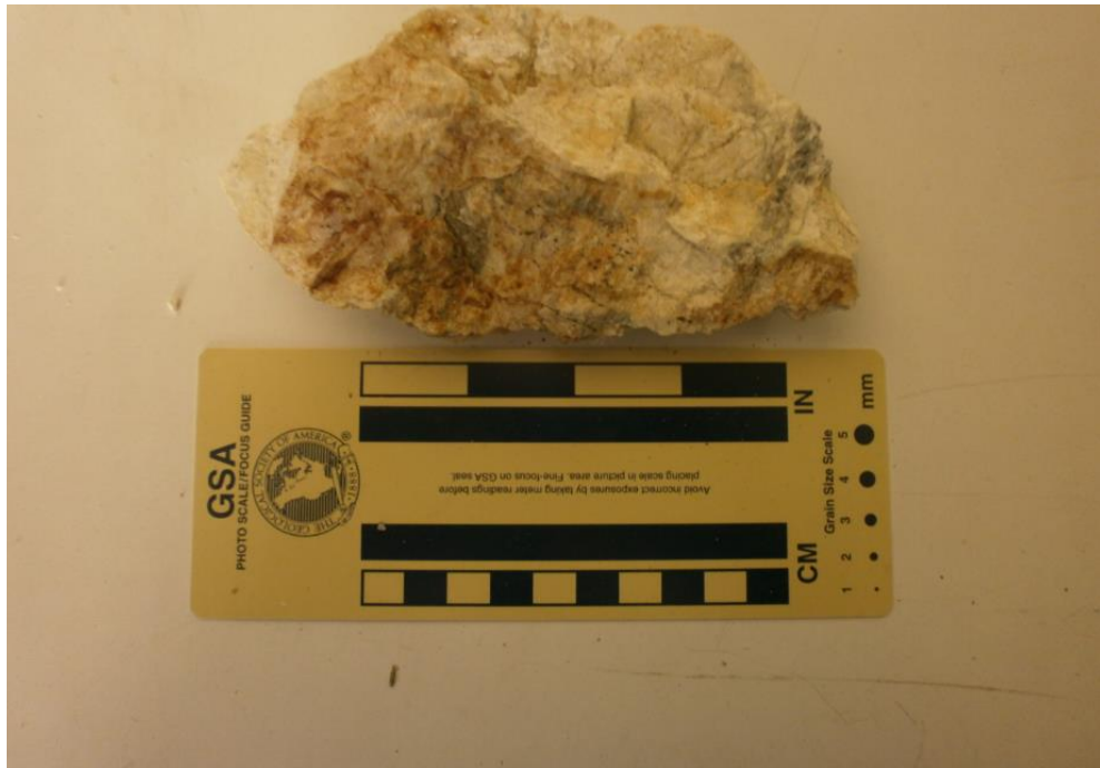
Figure 33. Rodingite sample (EROD18) with cataclastic texture and green colored chlorite veins.
