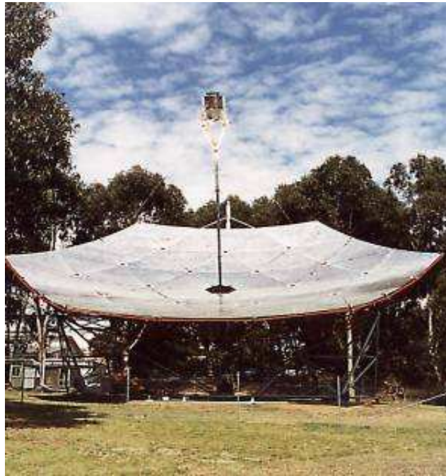
Figure 2.11: The big dish de 400 m 2 de l'Australian National University à Canberra[12]
