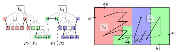
**Dynamic AMR in parallel.** Each color represents one of 1024 MPI ranks. The aggressive adaptivity required by the application results in 12 levels of difference in refinement, which corresponds to 3 orders of magnitude difference in cell size.
