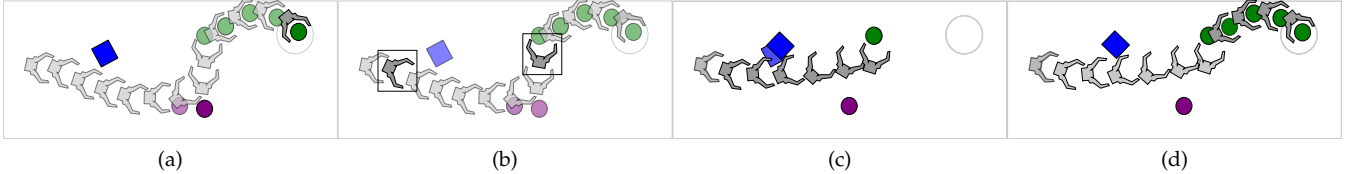
Fig. 3: The shortcutting algorithm. For simplicity, we depict only the motion of the end-effector. However, the whole arm is considered during planning. (a) The initial path. (b) The two manipulator states selected for connection. (c) The new states generated for the shortcut. (d) The new states added after the shortcut. The motion of the manipulator and green object remain unchanged. However, states are updated to reflect the new location of the blue box and purple circle.
