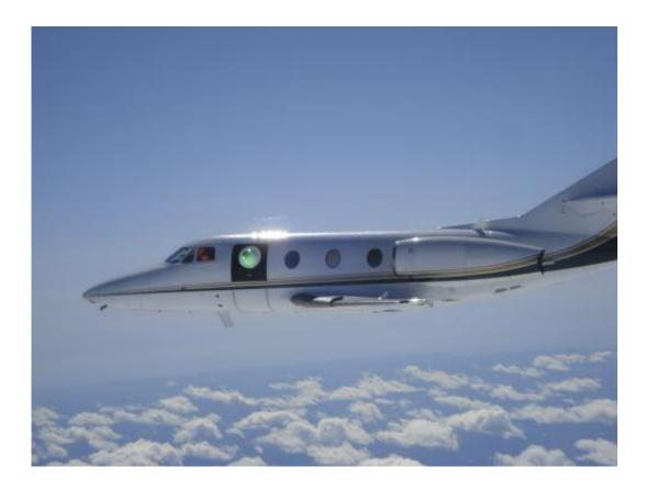
The Aero-adaptive Aero-optic Beam Control turret that Lockheed Martin is developing for the Defense Advanced Research Projects Agency and the Air Force Research Laboratory has completed initial flight testing. The prototype turret was tested on the University of Notre Dame's Airborne Aero Optical Laboratory Transonic Aircraft in Michigan. Credit: Air Force Research Laboratory
