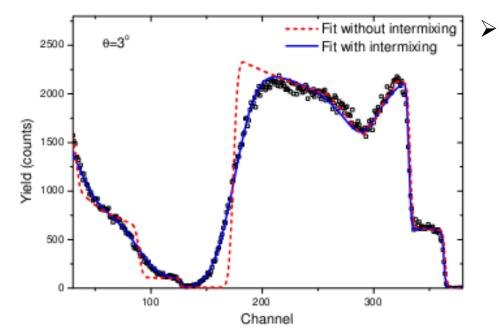
Film interacts with the substrate leading to extensive intermixing
