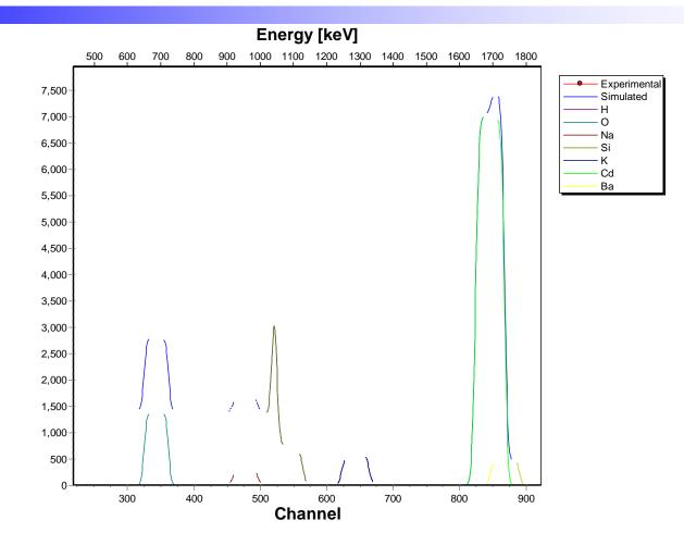
Substrate can be aligned to a major crystallographic direction to minimize background signal in some cases
