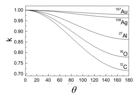
Plot of the kinematic factor, k, vs scattering angle for H<sup>+</sup> scattering from various targets
