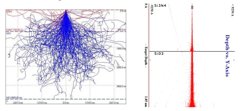
18keV e<sup>-</sup> and 18 keV He<sup>+</sup> striking a Si<sub>3</sub>N<sub>4</sub> layer with a SiO<sub>2</sub> substrate
