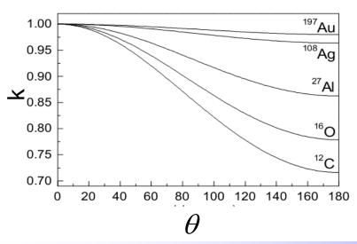
Optimized mass resolution for:  $160^{\circ} < \theta < 170^{\circ}$
