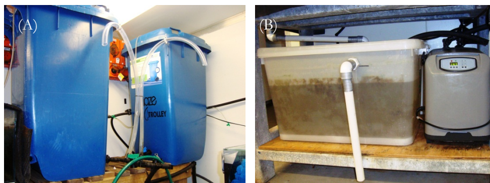
Figure 3. (A) Header supply system on egg incubation set-up for water disinfection. (B) Bio-filter/sump-chiller system on brood-stock tank.
