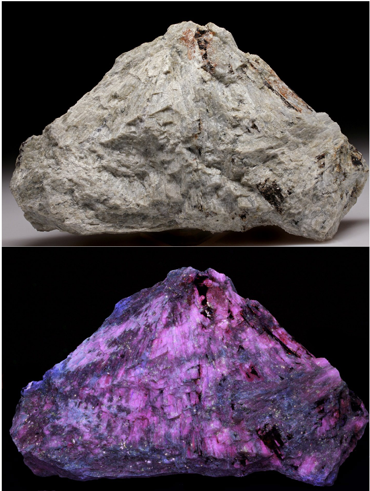
Figure 21. Mass of radiating marialite (based on Raman spectroscopy) 20 x 14 cm from a pod in altered lower marble member (Ssla) shown under normal light (top) and short-wave ultraviolet light (bottom). Dark areas in the top photo are pyrrhotite, which is also present in masses. (H. Moritz photos).
