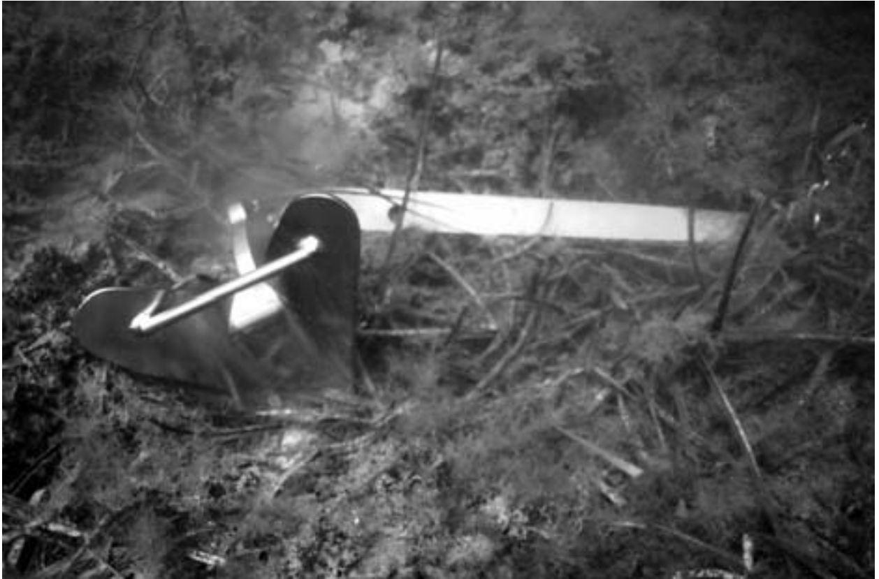
Figure 1.3—A ‘CQR’ anchor on a Posidonia oceanica bed at a depth of 10m. (For the color version of this figure please refer to the Annex at the end of the document)
