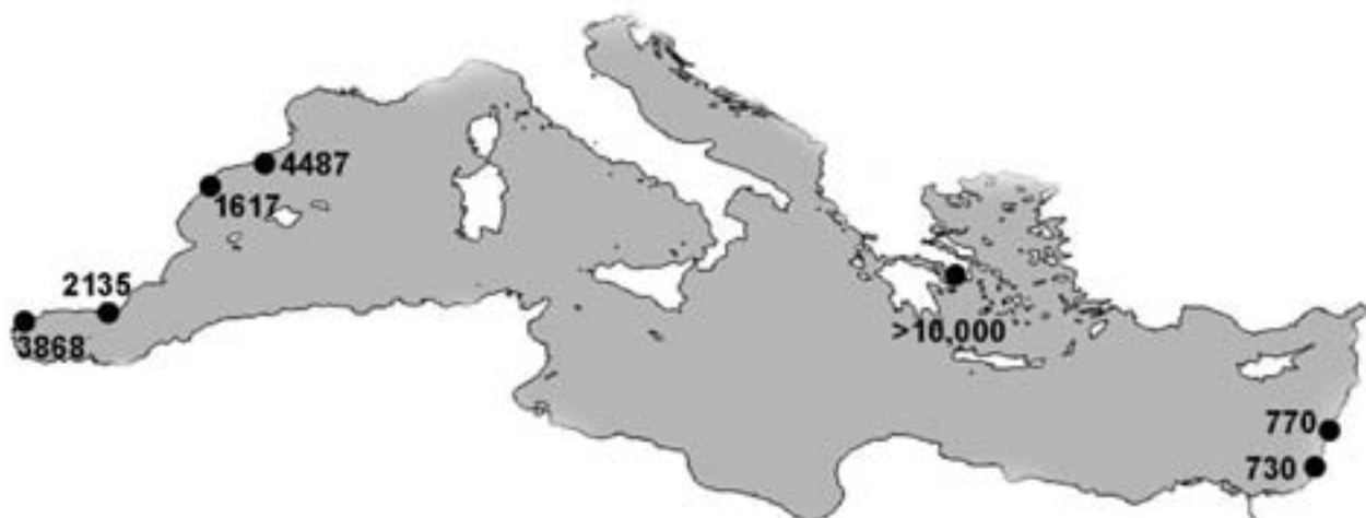
Figure 1.7—Concentrations of TBT in sediments ( \text{ng}\cdot\text{l}^{-1} dry weight) after the enactment of the ban on organotin-based antifouling paints in the Mediterranean in 1991. Sites sampled: Barcelona port, Almería port, Sotogrande marina, Sant Carles marina, Spain (Díez et al., 2002); Piraeus, Greece (Tselentis et al., 1999); Haifa port, Ashdod port, Israel (Herut et al., 2004; For the color version of this figure please refer to the Annex at the end of the document)
