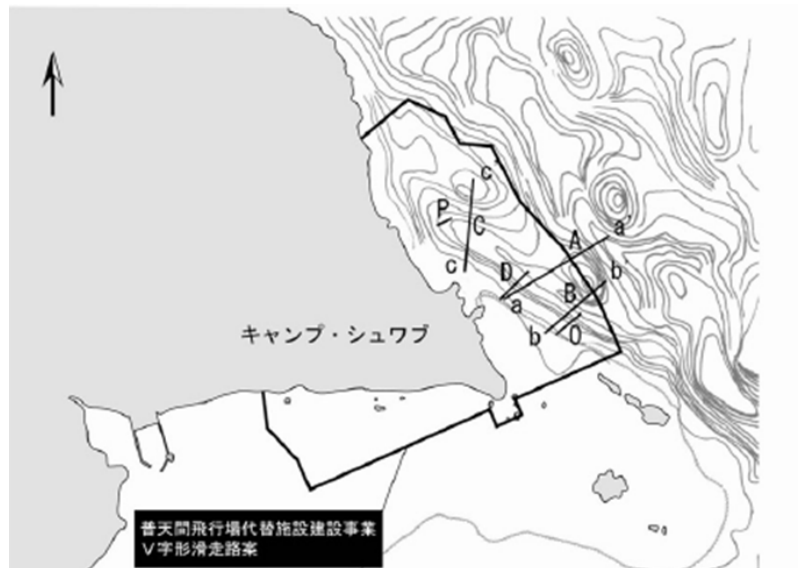
Figure 1. Seabed topography and survey transects in the reclamation zone.
