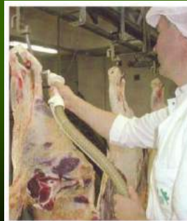
Fig. 1: Steam streams out from the suction head (beef carcasses)
