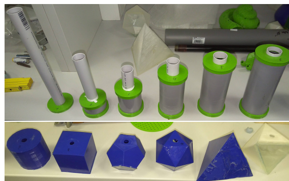
Figure 1: Built resonators: top - Morphed resonators (stepped-tube); and bottom - Platonic bodies (neckless resonators), numbered from left (1) to right (6).
