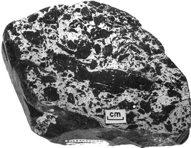
Figure 27.1-11. Sulphide-matrix (white) breccia ore with clasts of mafic metavolcanic wall rocks (black), Shebandowan, Ontario. GSC 203886-F
