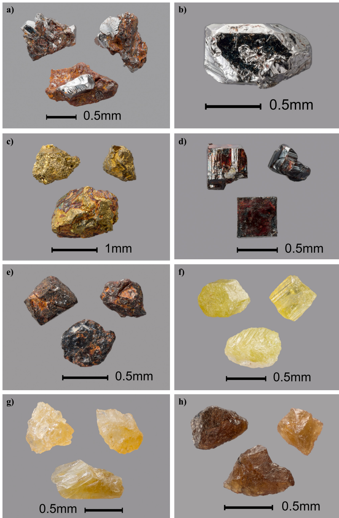
Figure 8. Colour photographs of indicator minerals: a) a small fragment of gossan sample 06-MPB-010 revealing sperrylite grains in a goethite matrix; b) sperrylite grain from till sample 06-MPB-011; c) chalcopyrite grains from till sample 06-MPB-027; d) pyrite grains from till sample 06-MPB-027; e) goethite grains from till sample 06-MPB-009; f) epidote grains from till sample 06-MPB-011; g) axinite grains from till sample 06-MPB-039; and h) titanite grains from till sample 06-MPB-011. Photos by Michael J. Bainbridge Photography.
