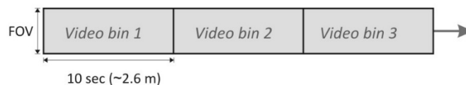
Figure 5. Schematic representation of video bins along a transect. Each bin can be viewed as a rectangle with width equal to the video camera's mean field of view (FOV; mean: 1.3 m) and length equal to distance ROV travelled over the 10-second interval (mean: 2.6 m).
