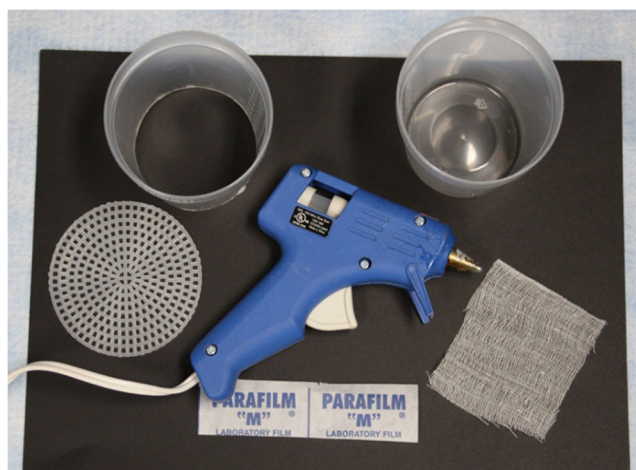
Figure G-1 Materials needed to construct a heat-extraction vessel; polypropylene 4.5-oz cups (2 per vessel), plastic mesh circle 14.6 cm, glue gun, cheesecloth, and Parafilm®.
