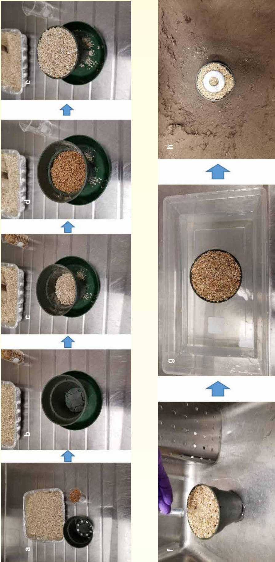
Figure C3. Assembling a Vernon bait trap: a) assemble materials - 10-centimetre (4-inch) pot, vermiculite, wheat seed; b) place pot in a tray (helps catch any spillage; c) fill first third of pot with vermiculite; d) fill next third with wheat seed; e) fill last third with vermiculite; f) saturate pot with water until water runs out of bottom of the pot - do this two times; g) place pot in a bin with several inches of water and allow pot to soak for 24 hours; h) dig a hole 5 to 15 centimetres (2 to 6 inches) deeper than the height of your pot, place the baitball at the bottom of the hole, bury the pot. Important: ensure soil is snug around the trap so there are no air pockets. Optional: add metal washer if using a metal detector to find the trap again. Leave for 1-2 weeks. Photos and descriptions: David Shack, AAFC-Lethbridge
