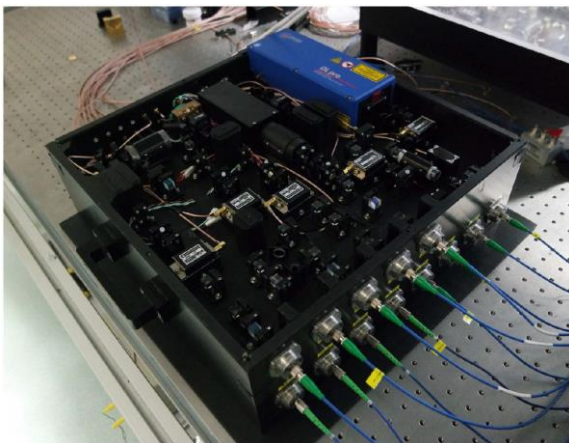
Fig. 24: Compact laser system for a fountain-type CAI gravimeter 21 .
