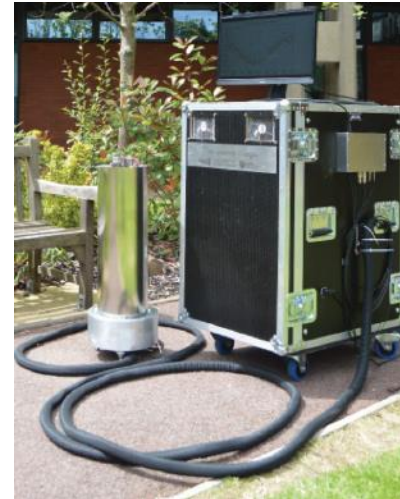
Fig. 27: Gravity gradiometer under development at Birmingham University 27 .
