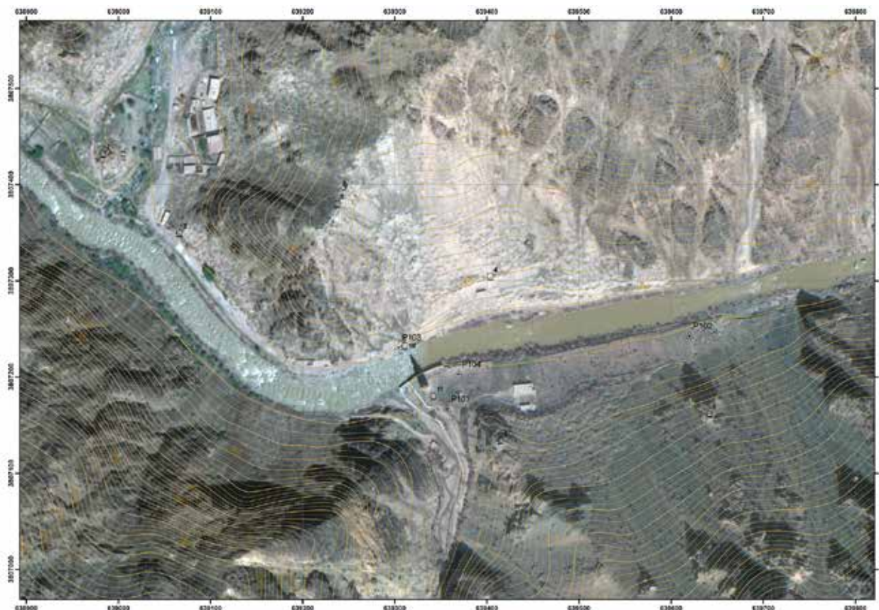
Figure 6. Extract of orthophoto map based on the fusion of two WorldView-2 images overlaid with topographic contour lines extracted from the Ikonos stereo-images (Image: by the Authors/DigitalGlobe).
