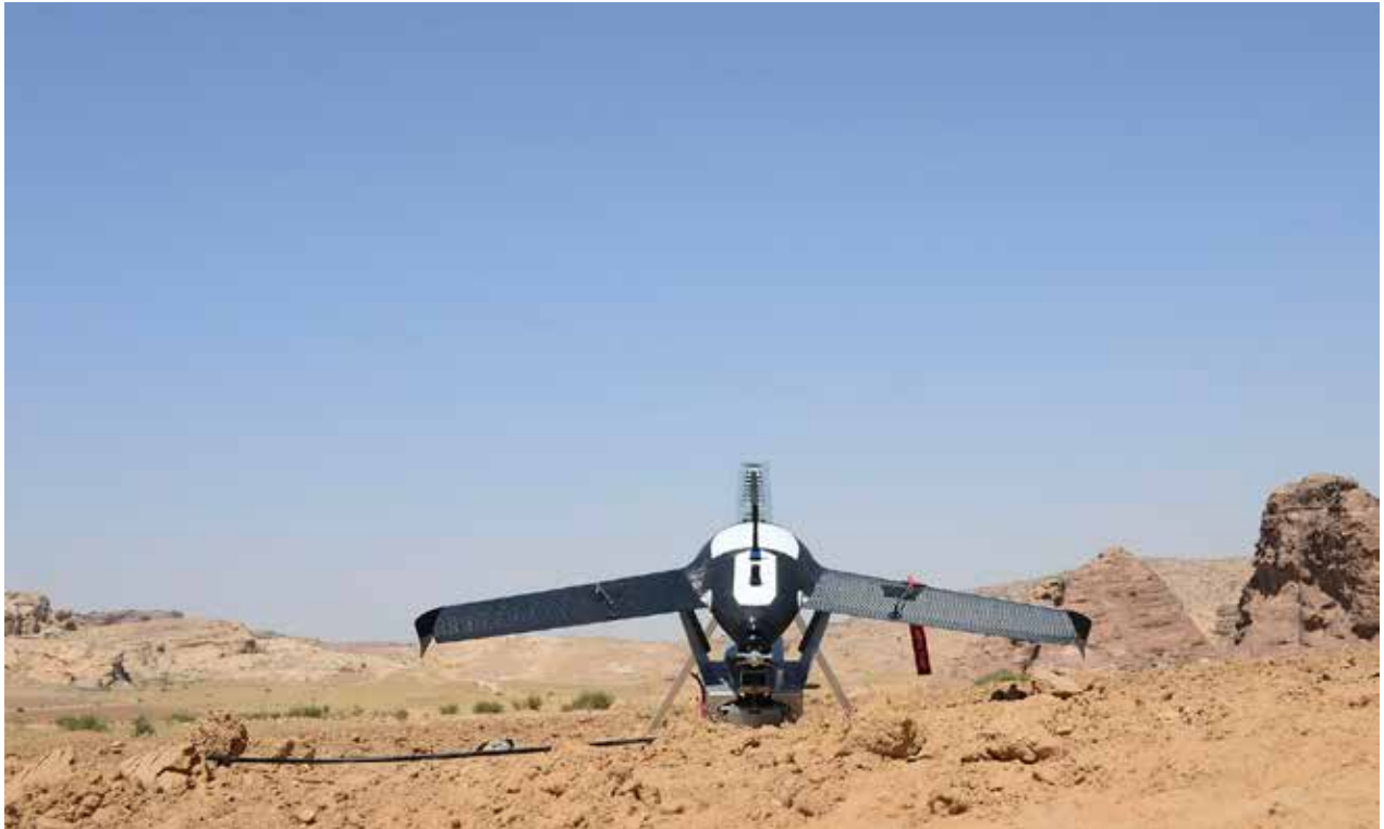
Figure 3. PPhoto of the Gatewing X100 fixed-wing UAS and catapult prior to take-off. The launch area was located approximately 2.5 kilometers northeast of the Ad Deir Plateau in the Al Beidha region. Photo courtesy of Bruce Allardice.
