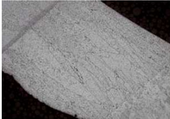
Fig 3.20 Aluminum weld showing assortment of microstructures in weld, base metal and heat affected zone. Etchant: 100 ml distilled water +2 ml hydrofluoric acid. Bright field, 100x.
