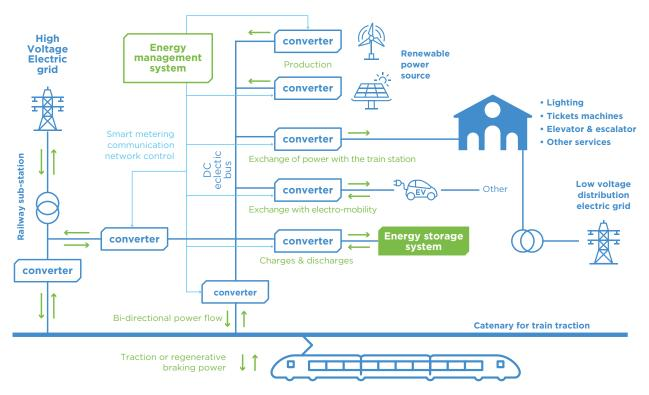
*Figure 31 / Schematic view of rail traction power supply in a smart power environment*
