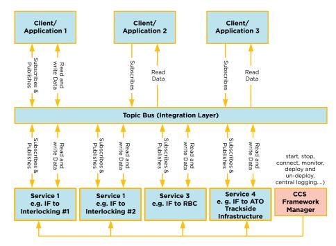
Figure 18 / Integration of different rail operation services
