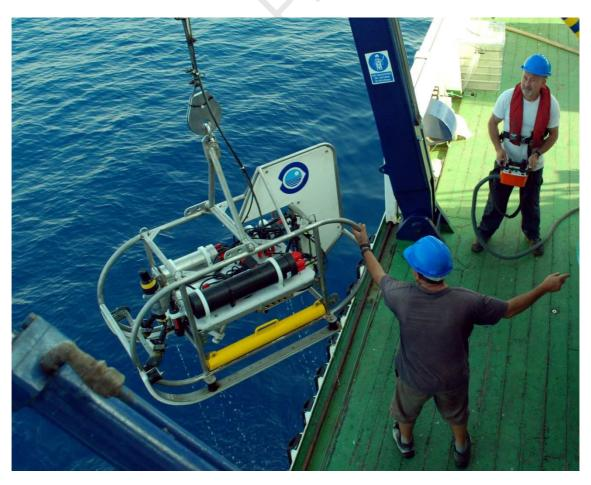
Figure 3. Politolana towed vehicle during its deployment maneuvers at the ECOMARG survey.
