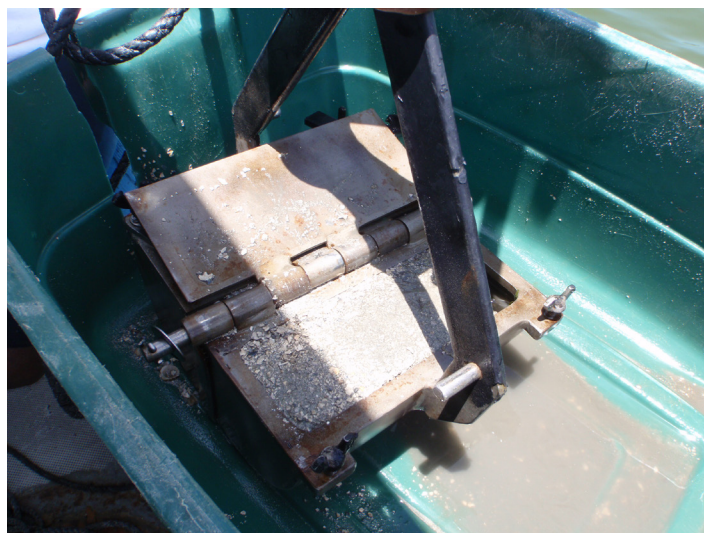
Figure 7. Image of the PONAR grab used to collect sediments in the SARI.
