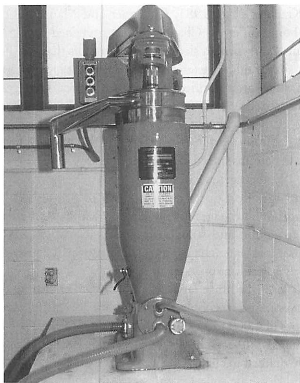
Figure 3. Sharples® centrifuge used to produce algal paste by separating algae from culture water
