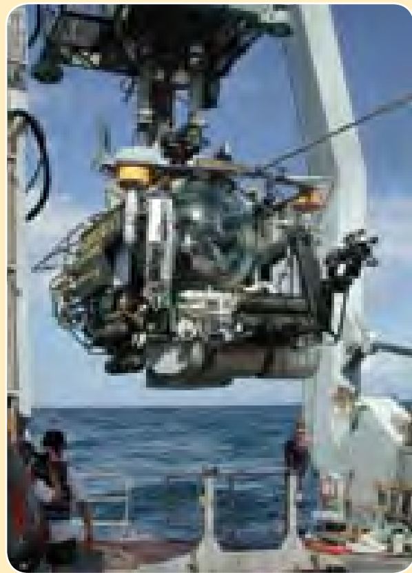
Launching of the Johnson-Sea-Link (JSL) 4-man submersible (2001). This is the primary tool used to collect benthic habitat data evaluated in this project. Photo credit: S.W. Ross et al.
