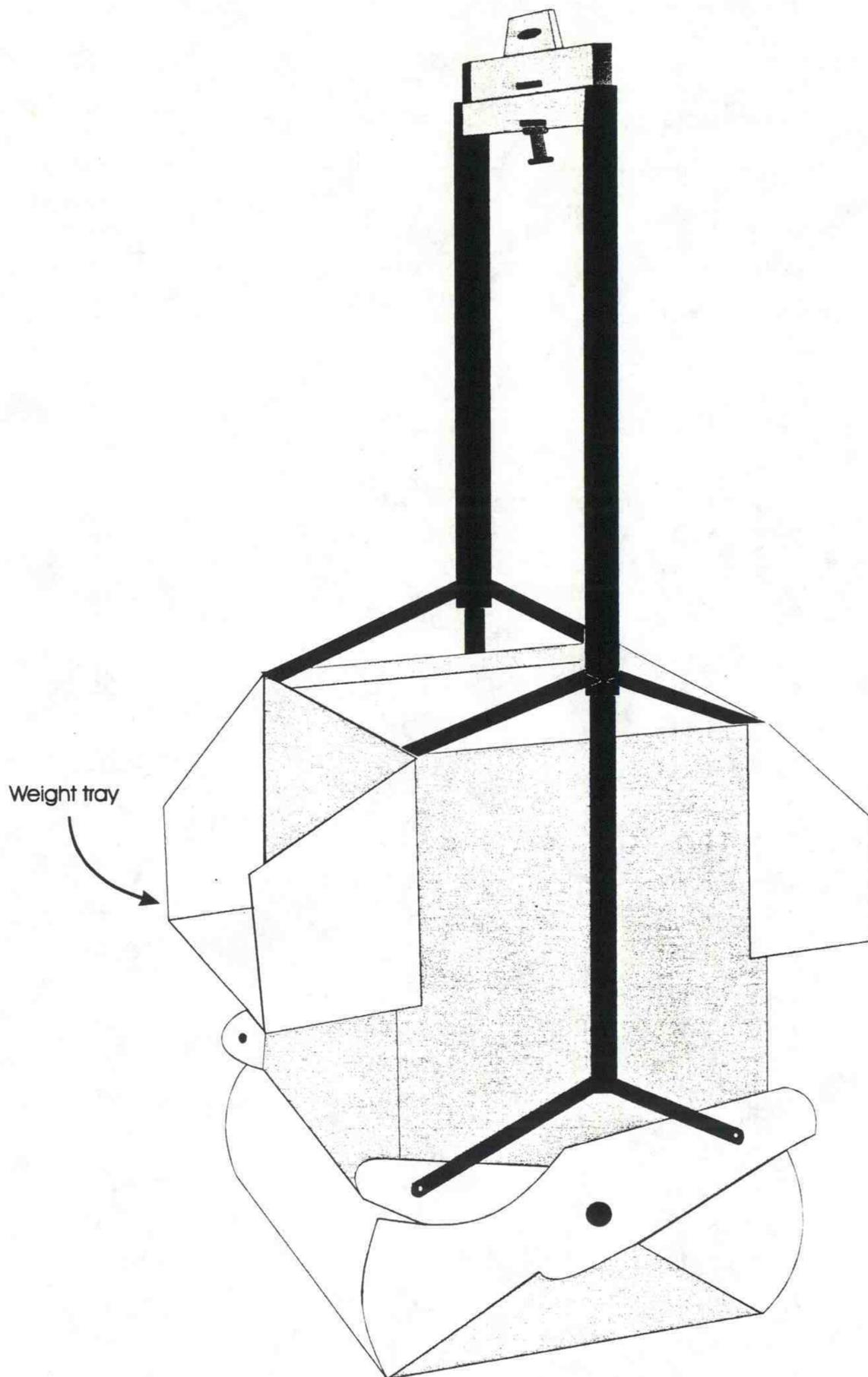
Appendix Figure 1. The 0.1-m<sup>2</sup> box corer (Gray-O'Hara modification of a standard box corer) used for benthic invertebrate sampling offshore from the Columbia River July 1993. For deeper penetration, 113-kg (250-lb) weights were placed in each tray located on opposite sides of the sampler.
