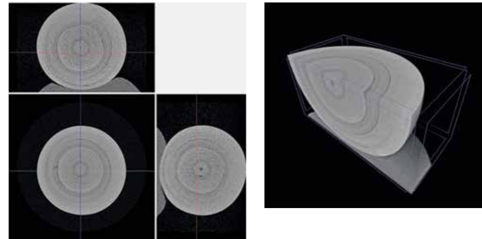
Fig. 2. Micro-CT images in the XYZ direction of the pearl depicted in Fig. 1, show concentric structures that confirm its natural origin.
