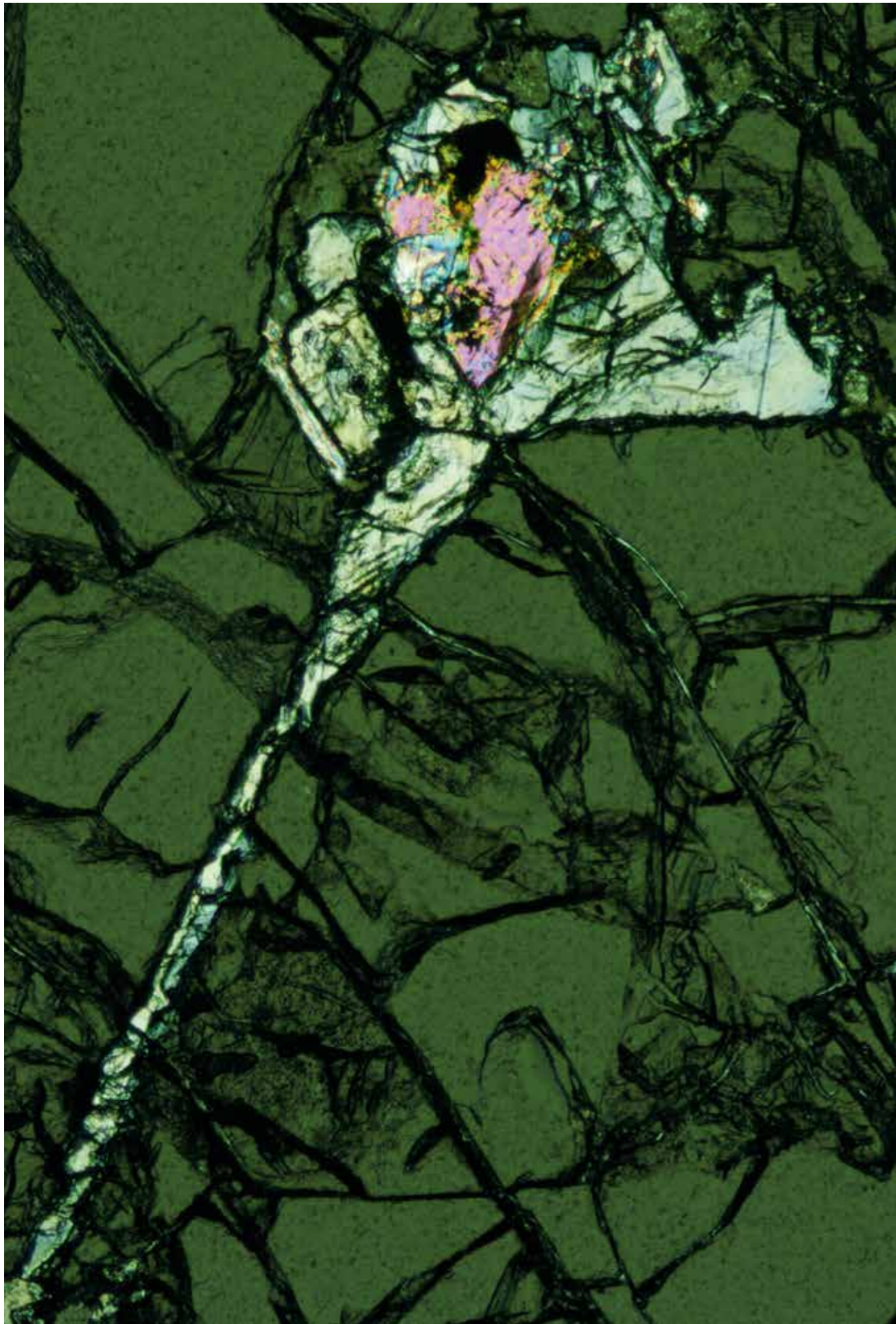
Fig. 1. Transmitted light microscopy image of a tulip-shaped corundum inclusion in spinel in a sapphire-bearing rock from eastern Sri Lanka. Width of view ~2 mm. Obliquely crossed (85°) polarized light.
