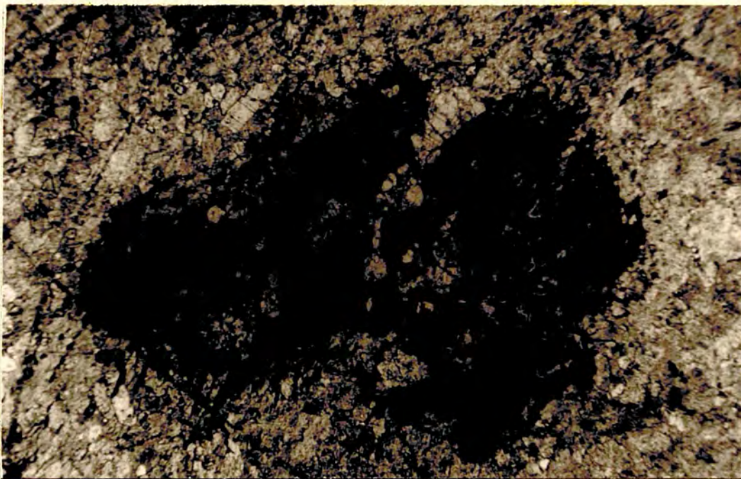
Plate 156. Pseudomorph, possibly after pyroxene, in the Ekiojango Carbonatite. (RF251). x55.
