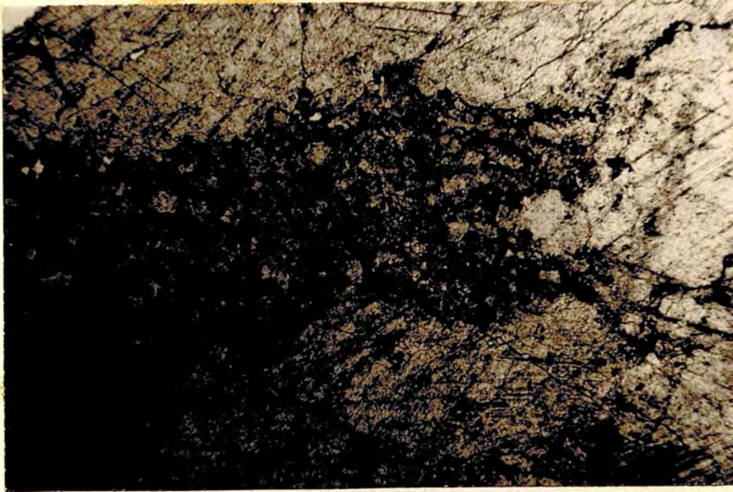
Plate 151. Fine-grained carbonate between large crystals of carbonate in the Ekiojango Carbonatite. (RF199). x25.
