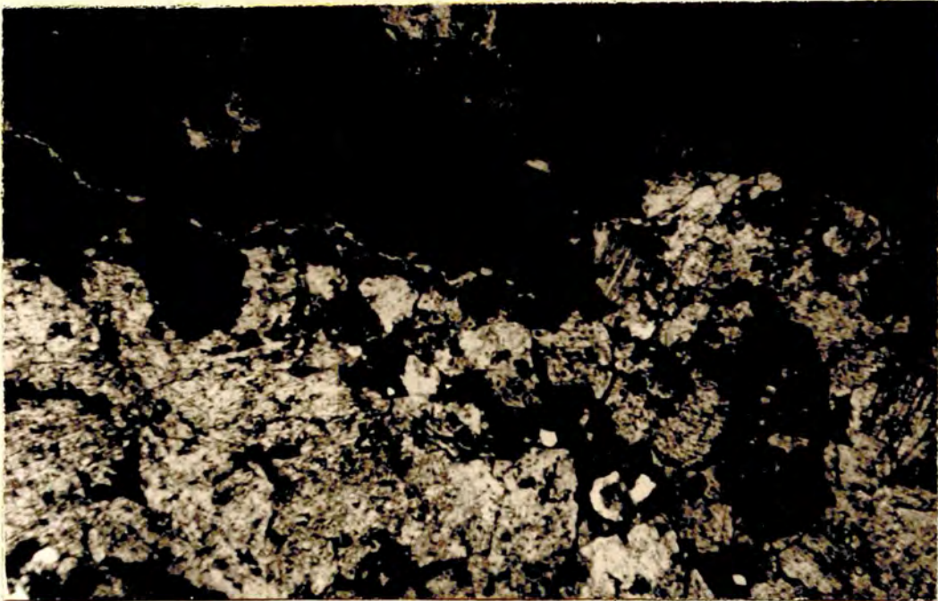
Plate 147. The contact at the edge of a carbonatite conesheet. The texture of the wall rock has been destroyed; the white material in it is fine-grained felspar. (RF44). x80.
