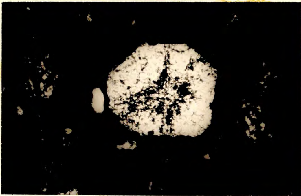
Plate 180. Pyrochlore crystal surrounded by ore in the Kinyamungu Carbonatite. (RF233). x80.
