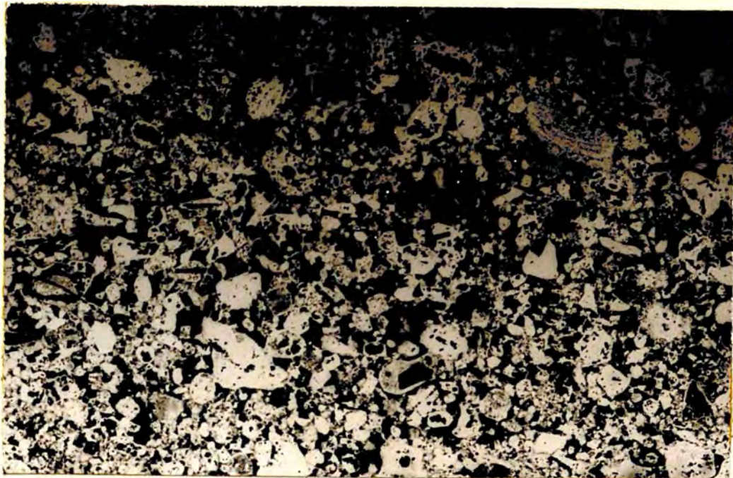
Plate 83. Typical texture of the Lower Agglomerate. Many of the fragments are themselves fragmental (negative). (RF147). x5.
