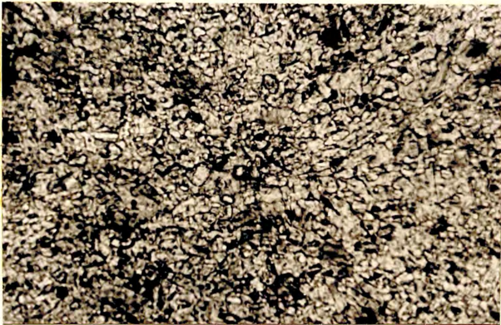
Plate 38. A felt of tiny crystals replacing melilite in altered biotite uncomphagrite. Possibly they are pyroxenes. (RFA33). x310.
