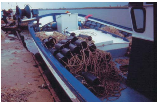
54) PVC pipe pots linked by a line for Octopus vulgaris fishery - Deltebre, Catalonia (M. Demestre)
