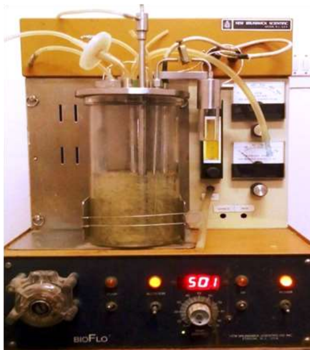
Fig.3.1 BioFlow C-32 New Brunswick Scientific, USA, fermenter used for the bioconversion of penicillin G to 6-APA using alginate entrapped penicillin acylase from Acremonium sclerotigenum
