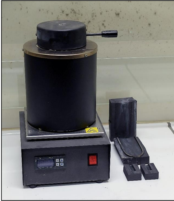
Fig. 4.3: Left: electric furnace with closed lid to minimise oxidation and on the right hand side the graphite ingot moulds.
