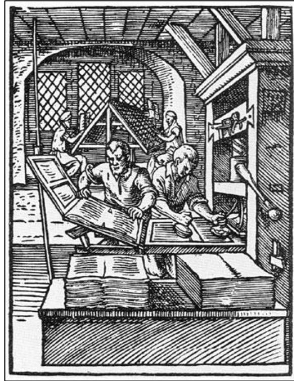
Fig. 1.2: Jost Amman 1568, a printing shop with compositors in the background, while co-workers are inking and changing paper at the press.
