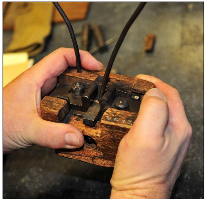
Fig. 1.13: A mould in the MPM collection, shown upside down, with the steel spring that holds the matrix in place.
