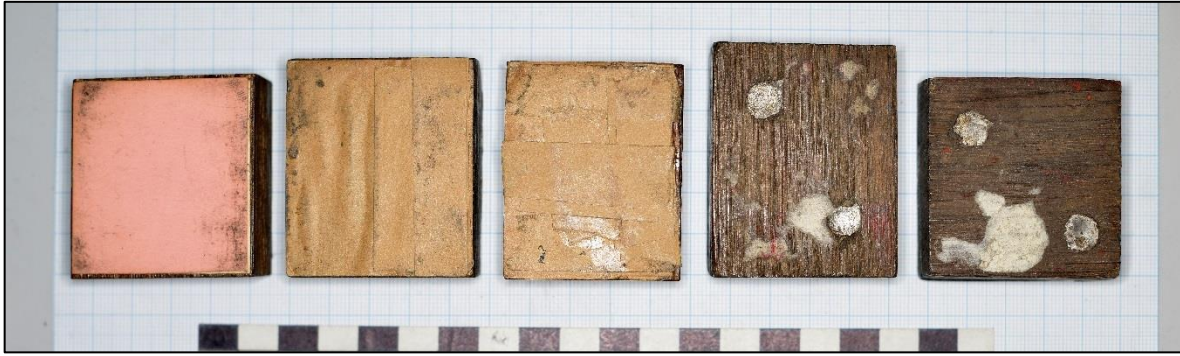
Fig. 4.29: Fronts, sides and backsides of the 5 measured printing blocks. While some are covered with paper at the back, others are free of paper and show the two drilled holes in the wood, which are filled with molten metal.
