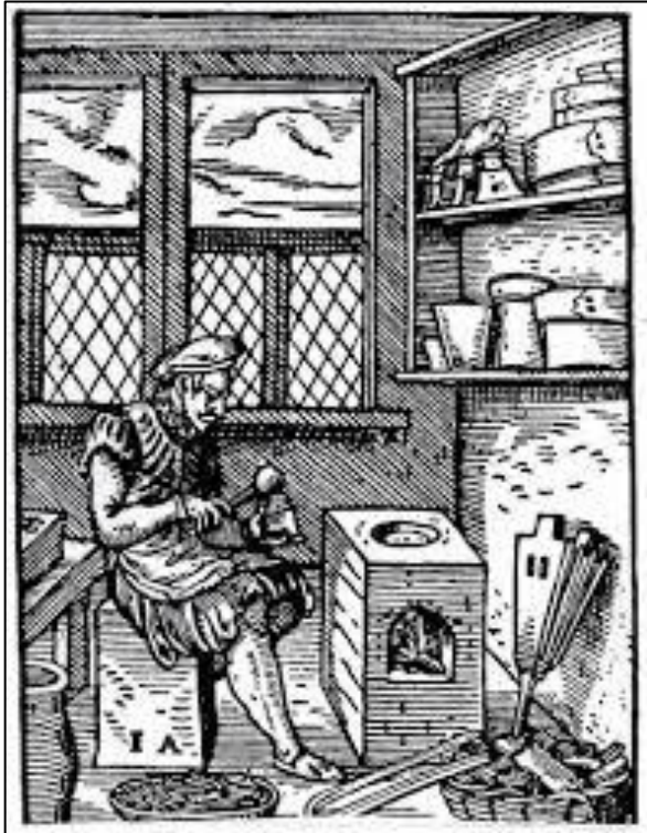
Fig. 1.1: Jost Amman 1568, a typefounder at work, casting a tin or lead alloy into a mould to make series of printing letters, collected in the basket on the floor.
