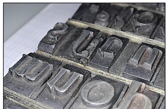
Fig. 4.34: Lead type cast from the wooden models above. The standing type composition with solitaire letters are respectively 12 x 15 and 12 x 17 cm large. The right image is a close-up.
