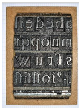
Fig. 4.34: Lead type cast from the wooden models above. The standing type composition with solitaire letters are respectively 12 x 15 and 12 x 17 cm large. The right image is a close-up.
