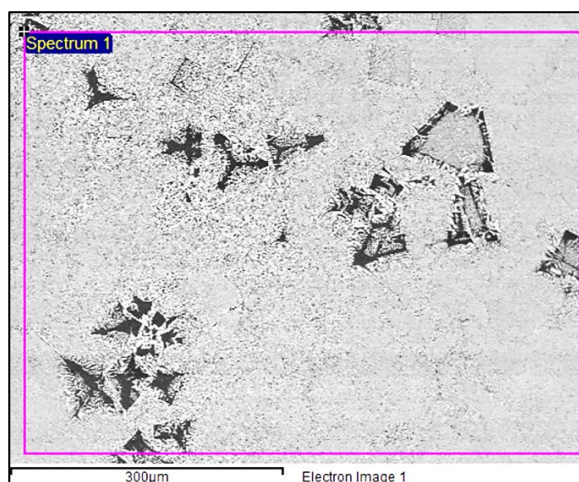
Fig. 4.15: Large area SEM-EDX measurement on alloy '76-12-12', approx. 600 x 400 \mu\text{m} (magnification of 500x, scale bar 300 \mu\text{m} ).
