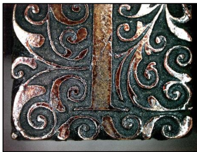
Fig. 4.66: Detail of one of the faces, showing remnants of ink and probably a lacquer coating.
