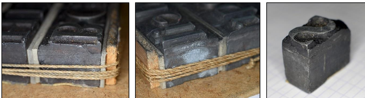
Fig. 4.35: Details of the sides show that the body was cast upon the face, which has an average thickness of about 4 mm.
