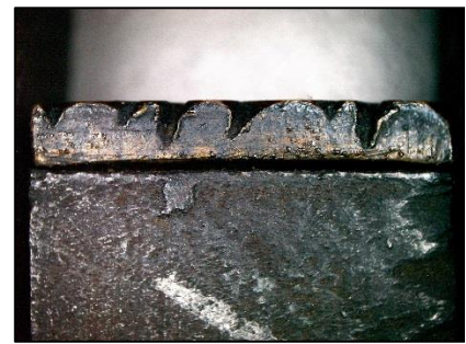
Fig. 4.68: Detail of the side, with burrs from engraving directly in the brass sheet.
