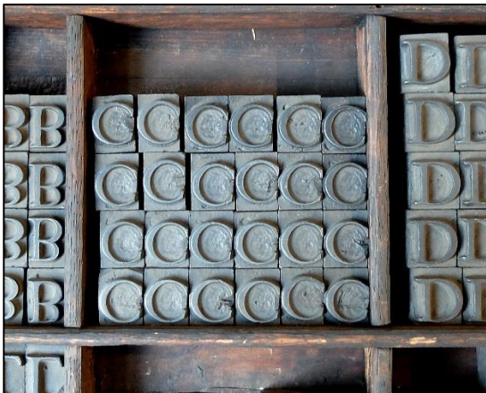
Fig. 4.41: Compartment of the exhibition case for the types 'C', cast on a high corpus.
