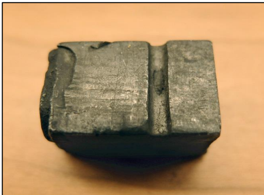
Fig. 4.58: One of the characters in cast lead, with the face wafer (left) and the cast-on shank.
