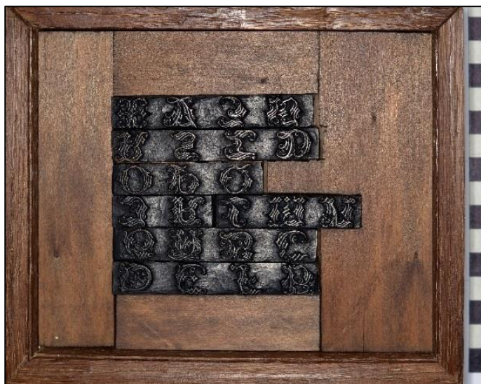
Fig. 4.53: Set of wooden characters, cut in pairs of 2, 3 and 4 on the same blocks.
