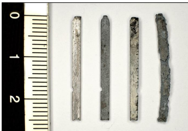
Fig. 6.1: Four types from left to right: without corrosion; with an even dark grey corrosion; with a dense white layer of passive corrosion and finally an example of a vigorously corroded item that has lost all structural rigidity, form and readability.
