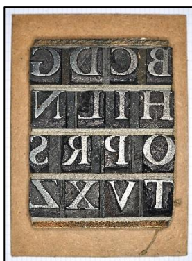
Fig. 4.34: Lead type cast from the wooden models above. The standing type composition with solitaire letters are respectively 12 x 15 and 12 x 17 cm large. The right image is a close-up.
