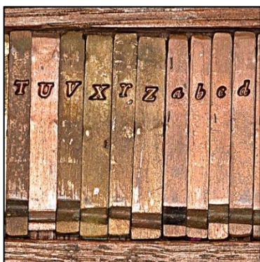
Fig. 5.13: Brass capitals T V X Y Z and copper matrices U, a-d.
