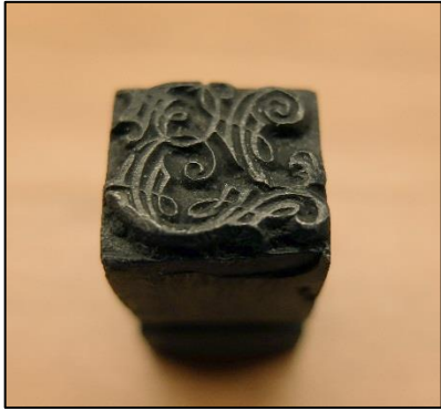
Fig. 4.55: Lead casting from the wooden models of ST 80.
