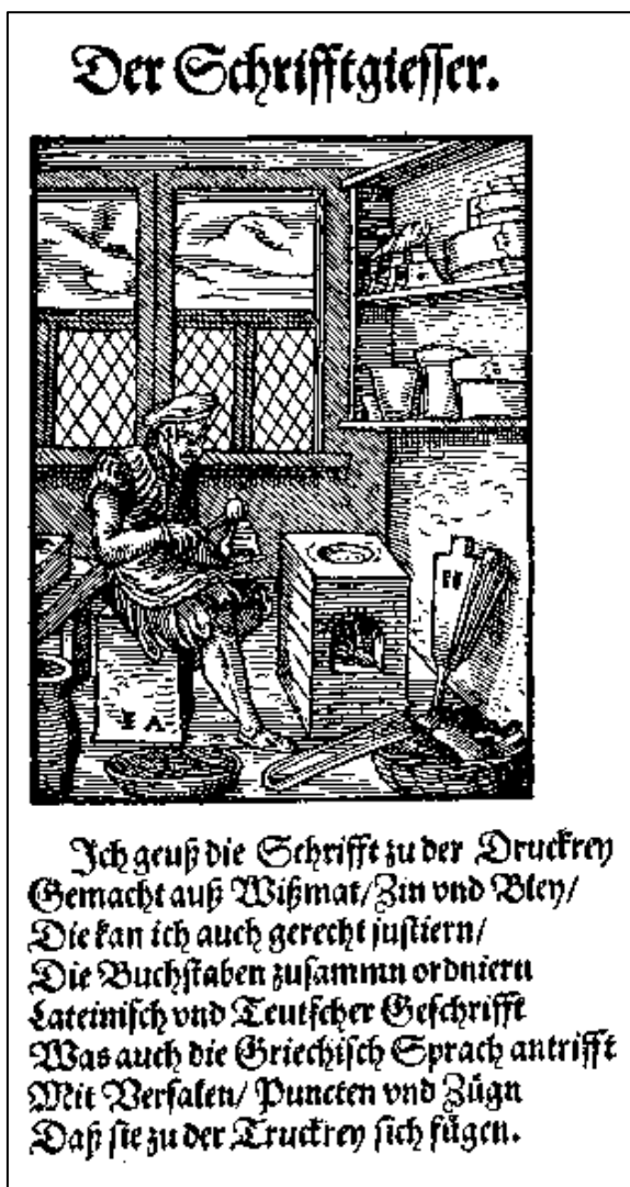
Fig. 2.8: Woodcut by Jost Amman, 'Beschreibung aller Stände', 1568: 2nd line mentions that the type metal is made with 'Wizmat/ Zin und Bley', being probably 'Bismuth, Tin and Lead'.
