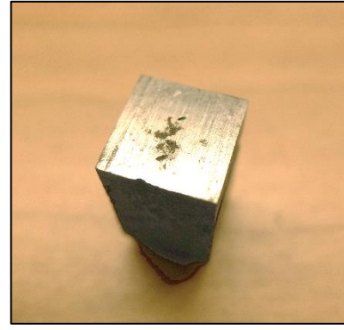
Fig. 4.57: Filed bottom of a shank with a shrinkage cavity*.
