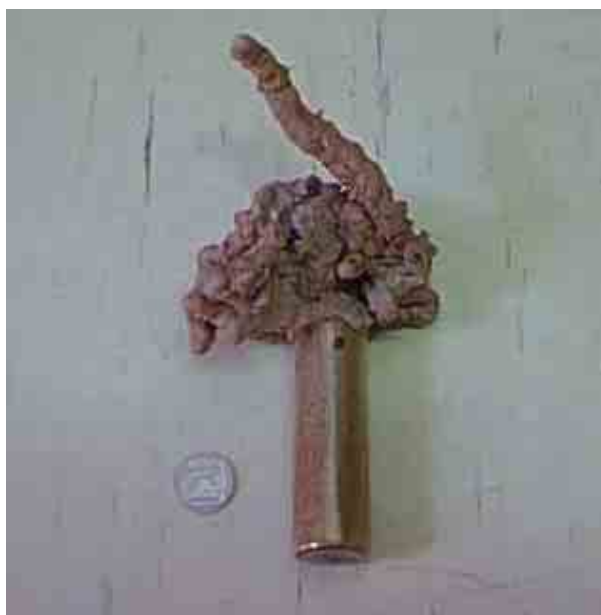
Figure 4-13 The same calcium gluconate sample after being heated at 300°C for 5 minutes
