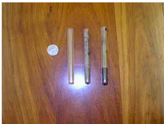
Figure 3-12 An empty glass tube (left) and tubes with pyrolysed samples (right) of the sodium salts
