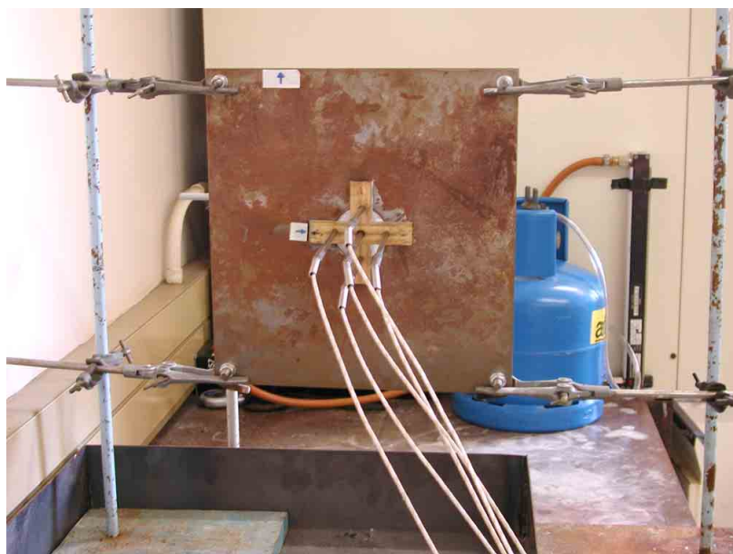
Figure 3-10 Back view of the burn test setup showing the thermocouples
