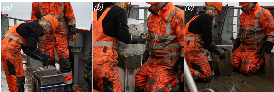
Figure S3: Retrieval of each intact core (LWH: 20 × 20 × 12 cm) obtained from (a) each of four replicate 0.1m 2 USNL (Unites States Naval Laboratory) box cores using a core extruder and (b-c), transferral to transparent acrylic aquaria (internal dimensions, LWH: 20 × 20 × 34 cm).
