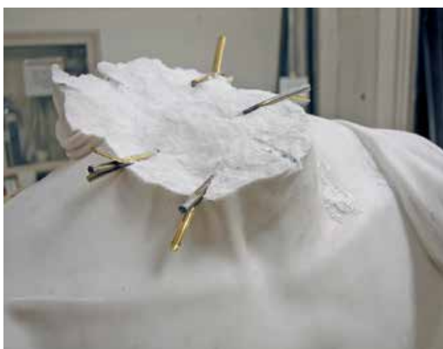
49a,b. Preparation of the David replica. Feathers and wedges were used to break the replica. This ancient method utilizes a series of drilled holes along the desired break line. Two “feathers” are placed into the holes, and then a metal wedge is inserted between the feathers. To break the stone, the wedges are tapped with a mallet so that a crack is propagated.
