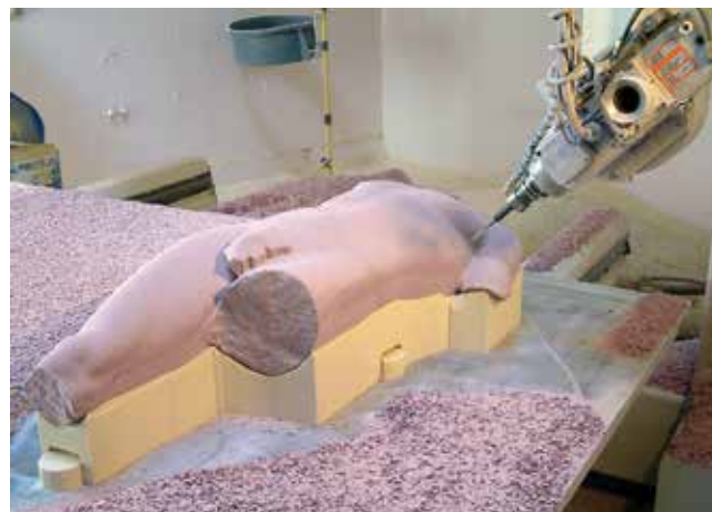
23a,b. Full-scale model of Adam's torso being fabricated in dense polyurethane foam by a computer numerically controlled (CNC) milling machine. This model was used as a mock-up to design the external armature as well as to formulate and rehearse assembly methods. Photographs: Ronald Street
