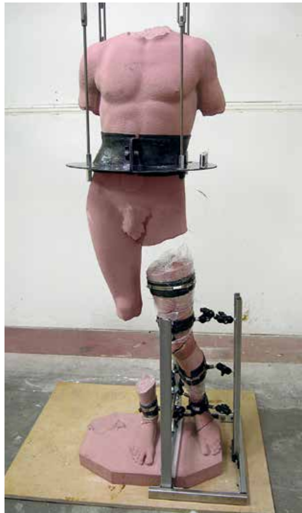
53. The full-scale milled model of Adam 's torso suspended over the left leg during armature development. The left leg is supported by carbon fiber straps and ball joints. The rigid support is constructed of metal strut channel framing stock.
