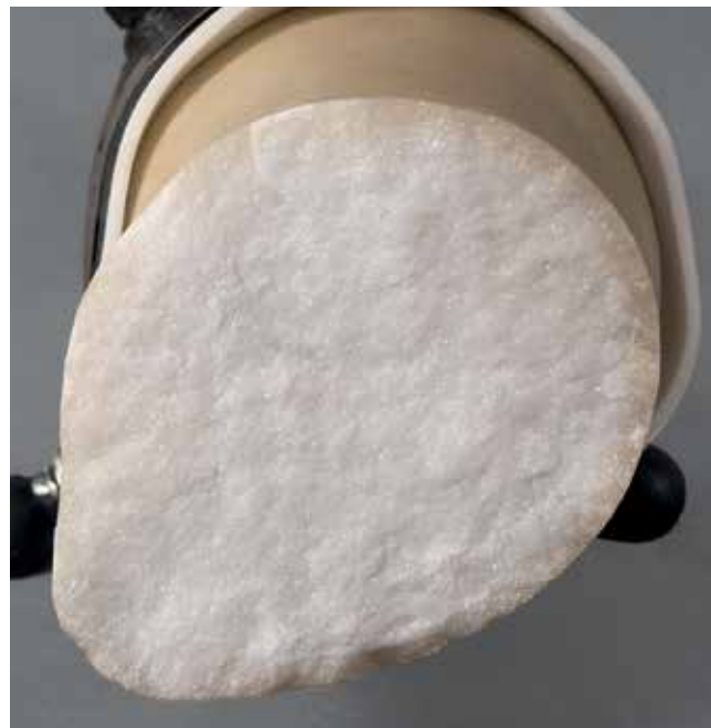
9. Fracture surface of the left calf fragment. This view of the interior surface illustrates the high quality of the Carrara marble, its pure white internal color, and its uniformity. The crisp break edge is in evidence, as well as past surface applications of fats that have penetrated the marble, visible as yellowing along the perimeter of the fragment.
