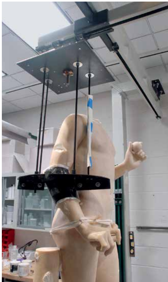
82. Assembly for attaching the right arm to the torso. This carbon fiber support strap was modeled after the torso corset. A flange extended from the strap to accommodate threaded rods that connected to an overhead steel plate. The entire assembly was suspended from the bridge crane, allowing lateral movement of the arm when required.
