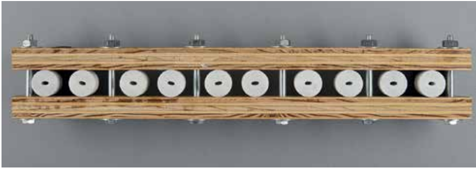
32. Preparation of Brazilian disk sandwiches. A clamping device was designed to mimic the maximum forces found in the sculpture. The specimens were left in the clamps for a minimum of three weeks while the adhesives set or cured.
