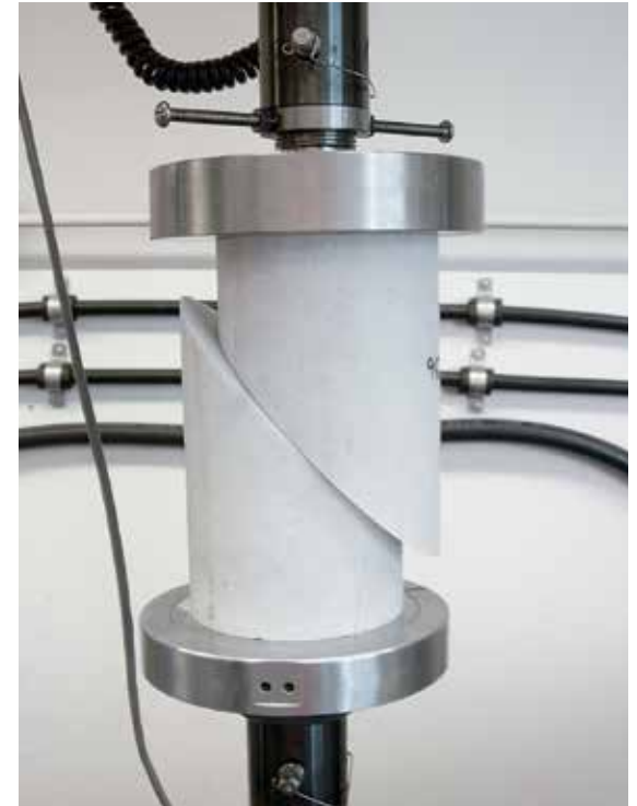
38. Testing setup for smooth-surface cylinders. The 8-inch-tall assembled specimens were subjected to gradually increasing downward force until there was failure of the pin or the marble. Photograph: Christina Muir
