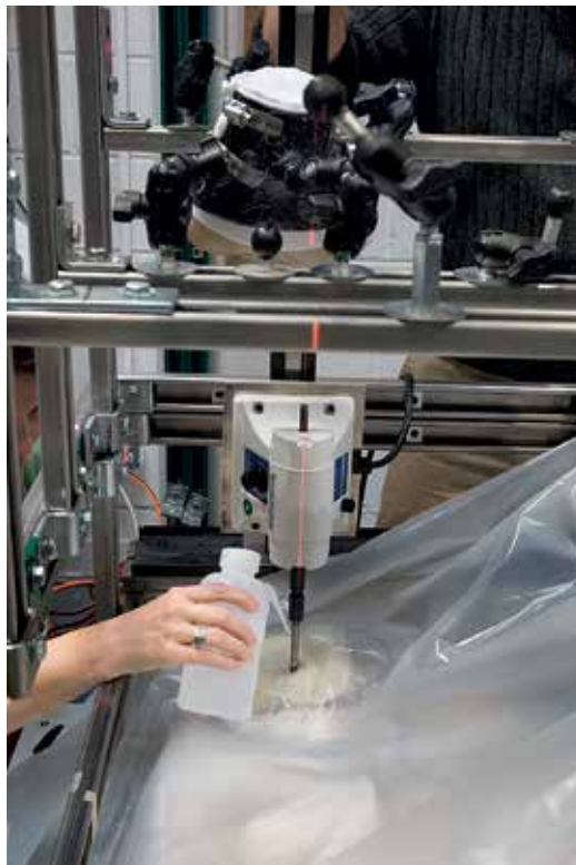
66a,b. Drilling the left ankle. Left: the pinhole is being drilled down into the base. Right: the corresponding pinhole is being drilled up into the left ankle fragment. Note that the drill is making a hole perpendicular to the base of the sculpture. Water was used to cool the diamond core bit and flush out the marble dust generated during drilling.
