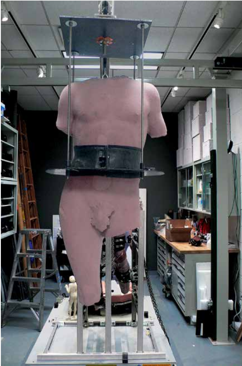
55. Completed torso corset for Adam . The torso was suspended by threaded rods from the overhead plate. Coupling nuts were turned to adjust the pitch of the torso. Adjustability was also designed into the suspension system, allowing fine pivot adjustments of the 380-pound fragment.
