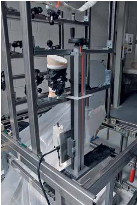
65. Alignment of the drilling device. Drilling was accomplished with a bench lathe turned on its side and attached to a linear actuator. In this illustration, the drill bit is attached to the lower axle of the bench lathe, prepared to drill downward into the base. The right ankle fragment is suspended above the drilling device.
