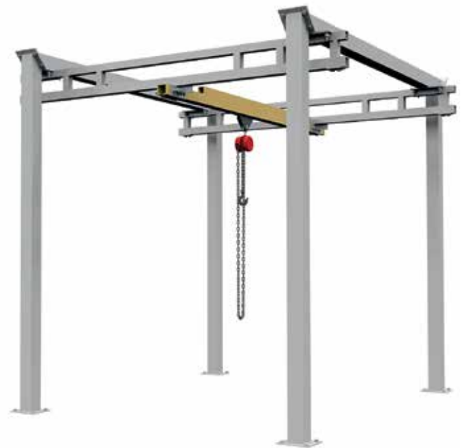
56. Freestanding bridge crane. An object can be positioned anywhere within the supports of the structure by means of the movable beam (highlighted in yellow). See also Figure 44.
