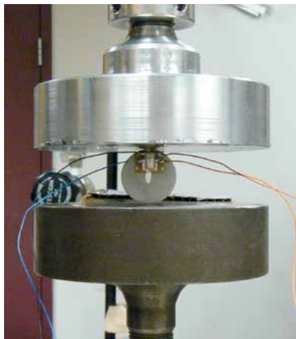
35. Creep testing setup. A foil gauge was applied to each specimen and then connected to a voltage meter that could detect small amounts of deformation. The load on the specimen was increased in stages until deformation was detected. Photograph: Andrea Buono
