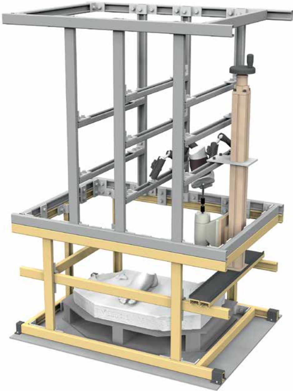
63. Ankle-drilling armature. With the rigid armature resting on the lift table, the ankle fragment was aligned to the base and locked in place with its ball joints. Next, the rigid armature was lifted to allow insertion of the riser (highlighted in yellow), providing space for the drilling assembly (highlighted in tan).
