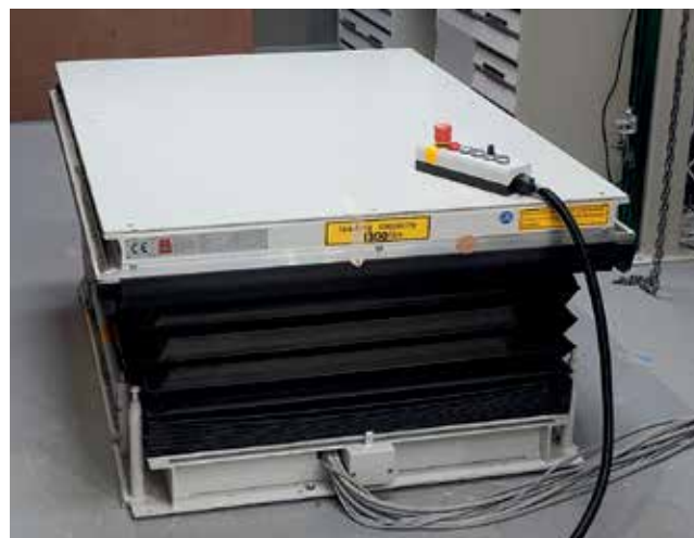
57. Lift table. This custom-designed piece of equipment was instrumental to the successful assembly of the sculpture. A remote controller allowed fine adjustments to the rate of the table's speed.
