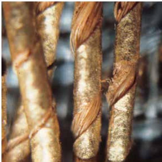
Appendix Figure 1. Metallic threads from the Saikyōji embroidery (Figure 7): paper strips gilded with the use of lacquer adhesive wound in a Z direction around silk S-Z core threads. Photograph: Masako Yoshida
