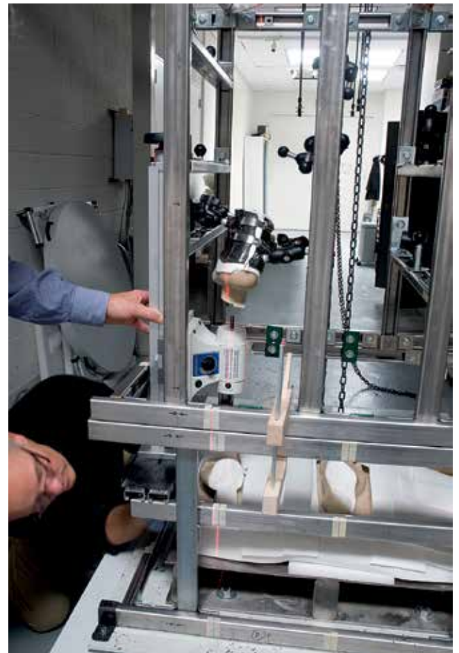
64a,b. Preparing to drill the left ankle. Top: the left ankle fragment rests on the base and the carbon fiber strap has been attached to the rigid framework, locking in its alignment. Bottom: the left ankle fragment is suspended in the armature after insertion of the riser. Red laser lines projected onto the armature were essential to maintain alignment of the fragments.
