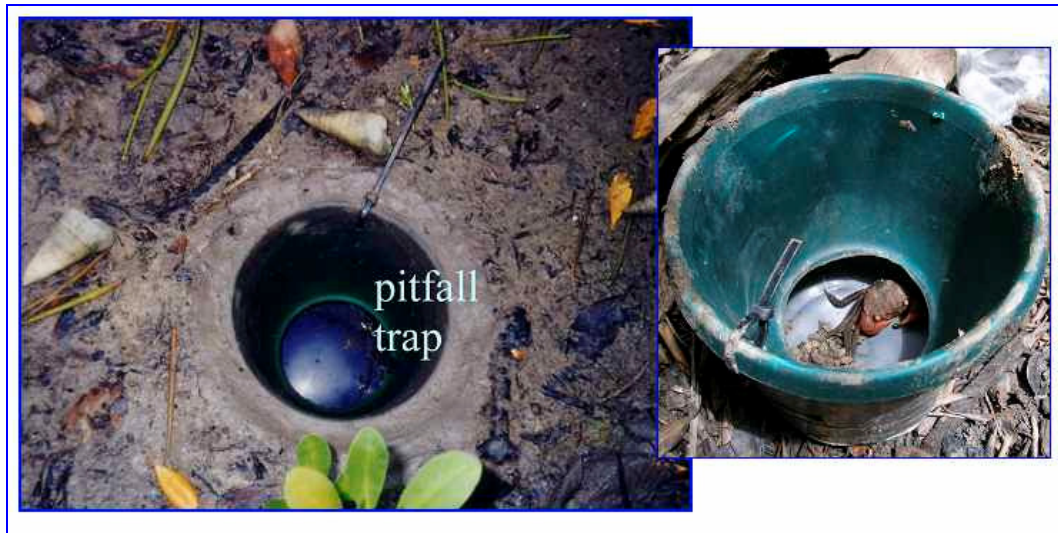
Figure 5-4: Mangrove pitfall trap for sampling mobile, nocturnal and puddle fauna. Inset: The collar prevents crabs, such as Neosarmatium meinerti pictured, from escaping.
