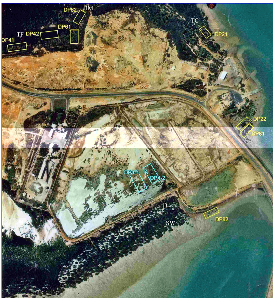
Figure 2-8: Aerial photo of the East Arm Port facility under construction in 2000, indicating location of 25 m ×100 m study sites in four mangrove assemblages (where SW = seaward, TC = tidal creek, TF = tidal flat and HM =hinterland margin.) During 2001 the remaining seaward mangroves (lower left) were also cleared.
