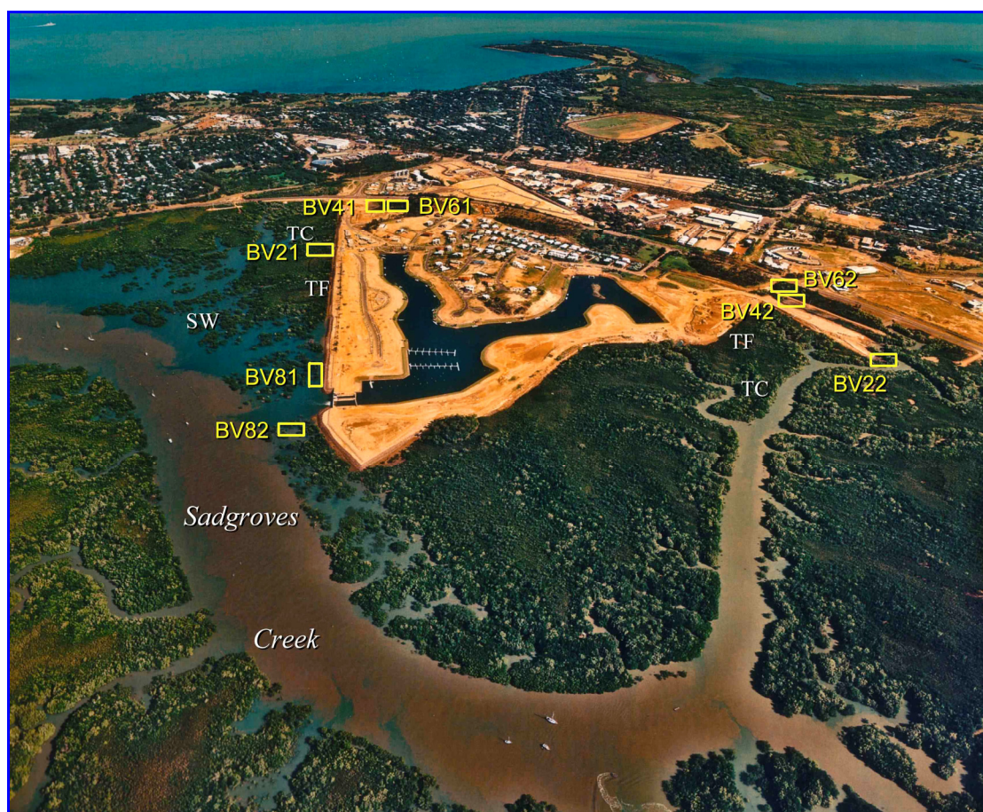
Figure 2-7: Aerial photo of Bayview residential and marina development under construction in May 2000, indicating location of 33 m × 75 m study plots in four mangrove assemblages. The high turbidity evident in Sadgroves Creek (foreground) is presumably inwashed terrigenous sediments from earthworks and clearing of vegetation within the catchment.
