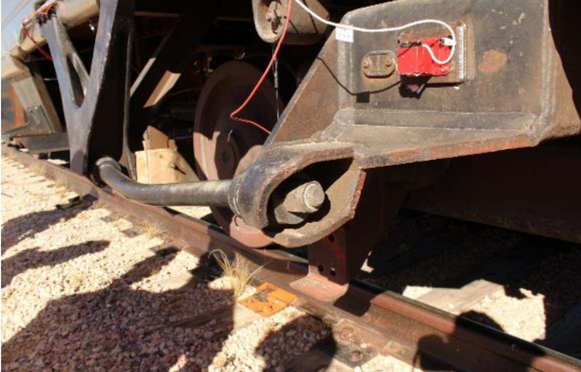
Figure 99. Bent Traction Rod after Third Test
