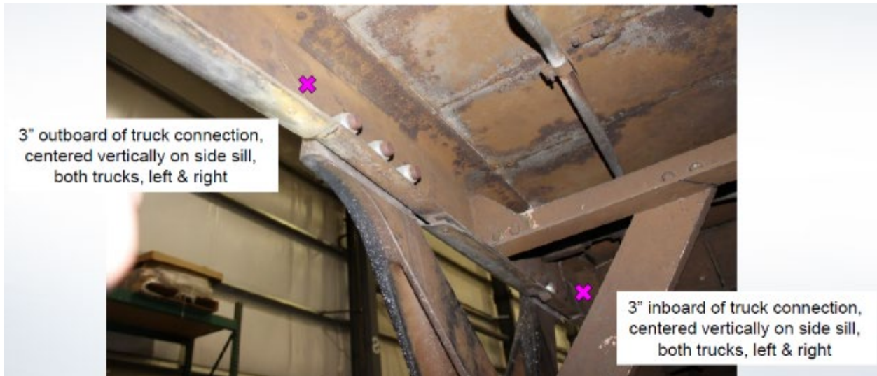
Figure 24. Strain Gage Locations on M1 Passenger Car
