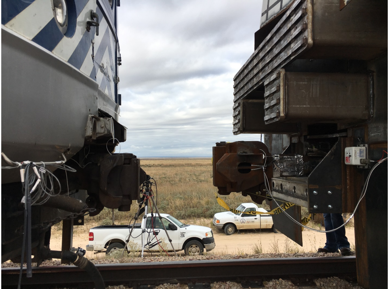
Figure 3. Initial Coupler Misalignment
