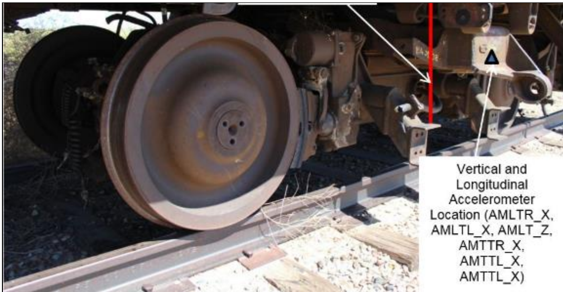
Figure 19. String Potentiometer and Accelerometer on M1 Passenger Car Truck
