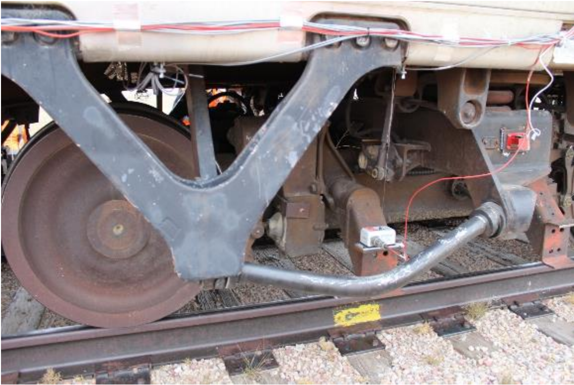
Figure 101. Bent Traction Rod after Fifth Test
