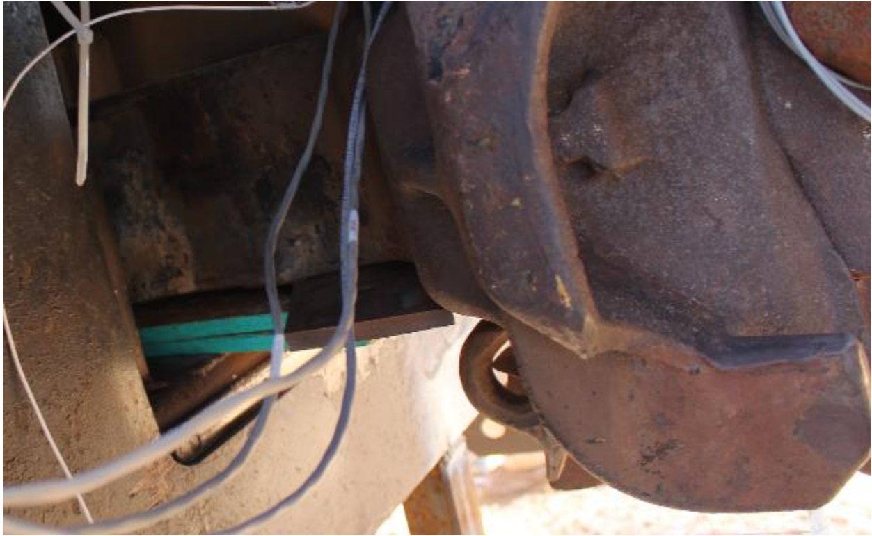
Figure 5. Coupler Carrier and Shims on the M1 Car
