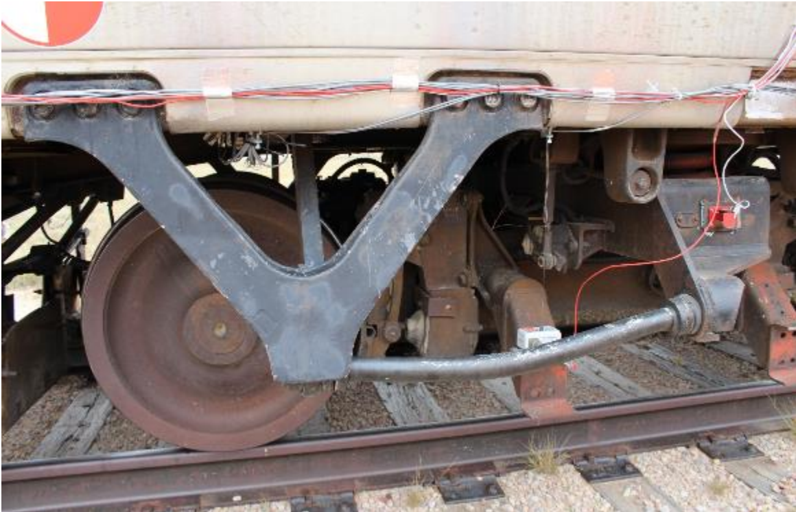
Figure 100. Bent Traction Rod after Fourth Test
