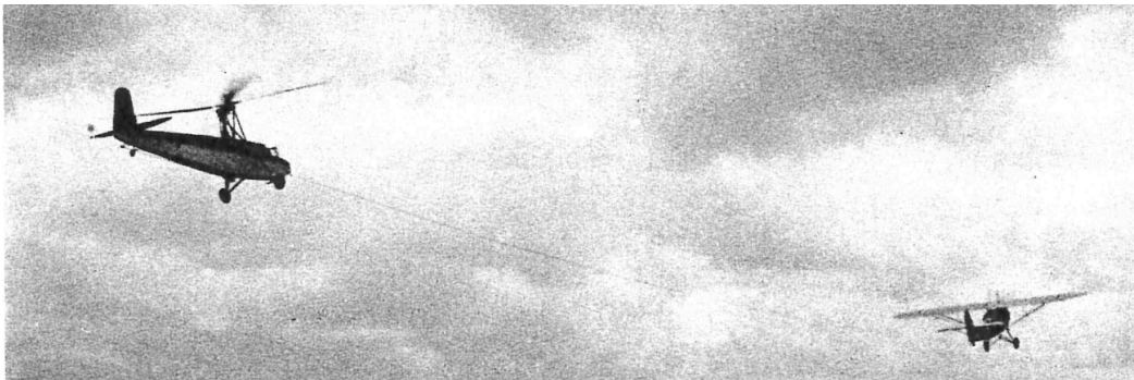
Fig. 26: Gyrocopter towed by a He 46
