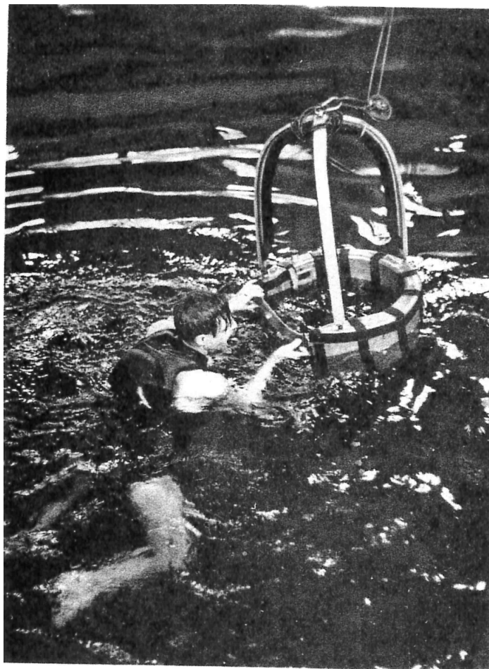
Fig. 36: Lift cage for Fa 223 - sea rescue aircraft
