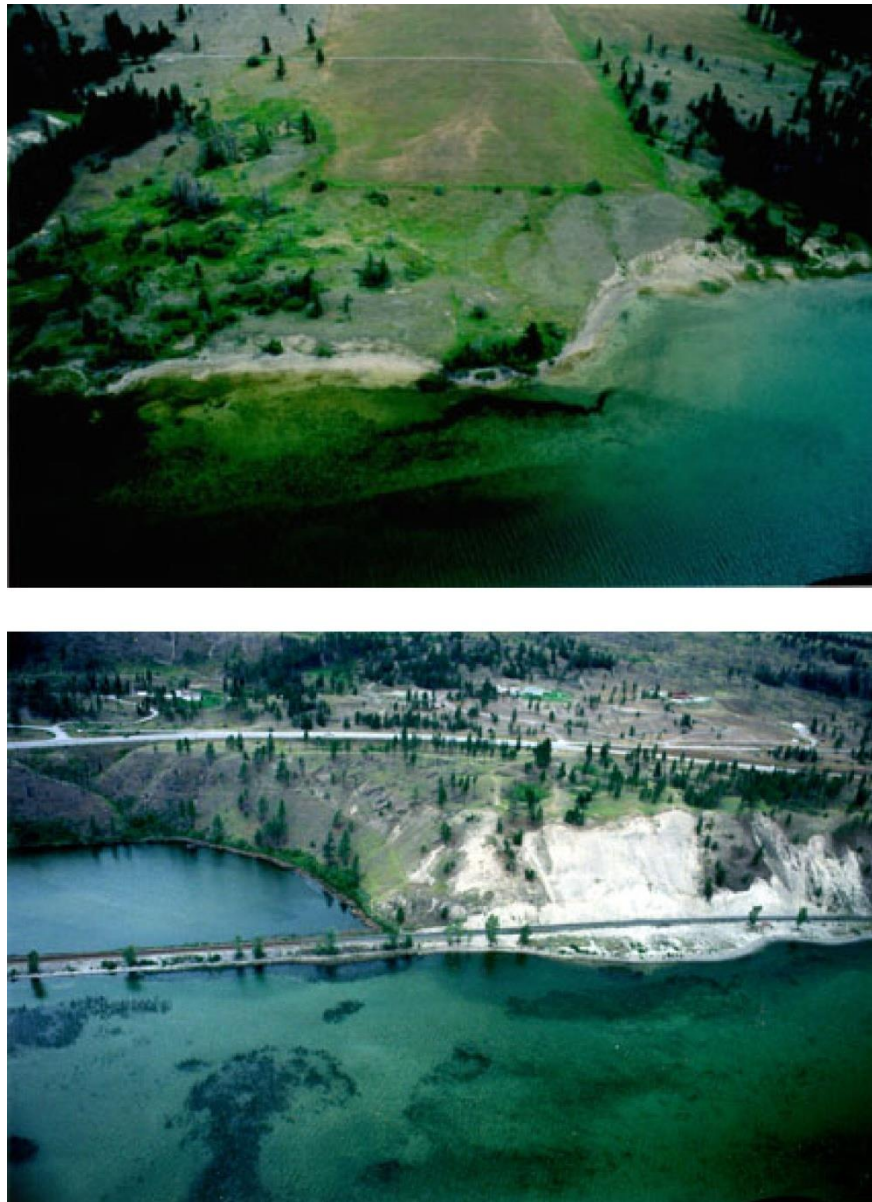
Figure 11. Columbia Lake showing unmodified shoreline (upper) and shoreline modified by riprap of a railway corridor (lower).
