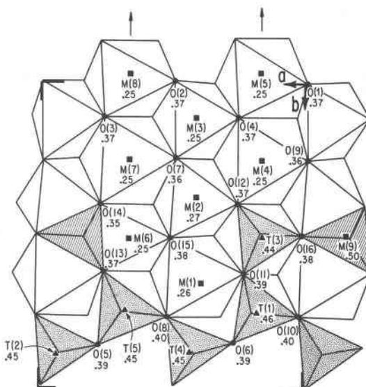
Fig. 1. Polyhedral diagram of the surinamite structure down  $z^*$  between  $0 < z < 1/2$ . Octahedra in the walls are unshaded and the tetrahedra are stippled. The M(9) octahedron between the walls resides above the ruled region. Compare with Fig. 1 in Moore (1969).
