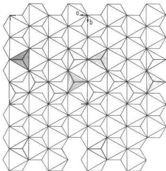
Fig. 2. Idealized polyhedral diagram of the surinamite crystal structure down  $z^*$ . The octahedral walls are unshaded, the (Si,Al)-O tetrahedra are stippled and the Be (= T(1))-O tetrahedra are ruled. The M(9) octahedra between the walls reside above the shaded regions. Tetrahedra below the walls are not shown. The surinamite cell is outlined.
